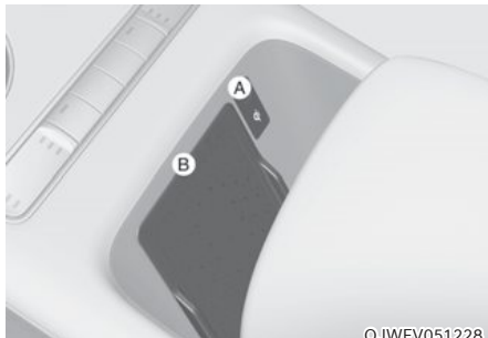
[A] : Indicator light, [B] : Charging pad
