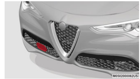
Front fascia/bumper Radar Location
