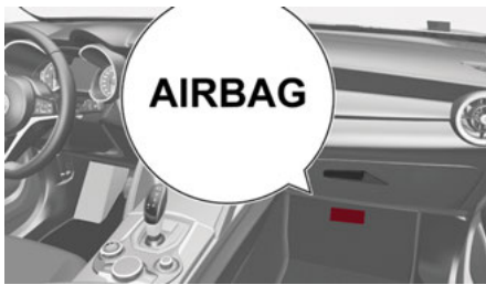
Passenger Knee Air Bag Location/Knee Bolster Location
