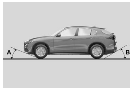
Front And Rear Loading Angles
