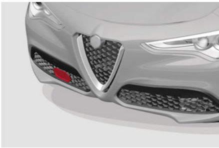
Front Bumper Radar Location
