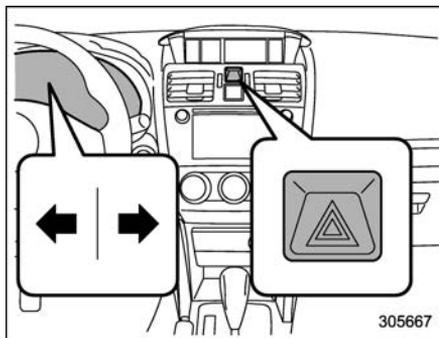
Use the hazard warning flasher to warn other drivers when you have to park your vehicle under emergency conditions. The hazard warning flasher works regardless of the position of the ignition switch.
