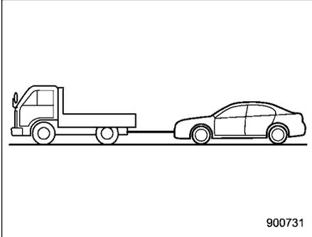
1. Release the parking brake and put the transmission in the "N"/neutral position.
