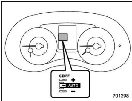
In the auto mode, the system estimates the driving and road conditions using signals from the wheel speed sensor, throttle position sensor, steering angle sensor and brake switch, etc. According to the result, it electronically and automatically controls the degree of limitation of the differential action (LSD torque) to optimize the differential action of the center differential. When you turn the ignition switch ON, the "AUTO" indicator on the combination meter appears.
