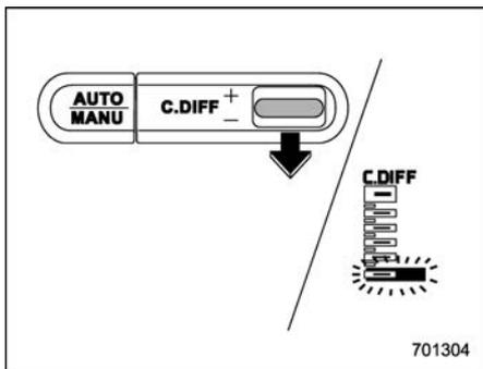
Pull the switch rearward to reduce the initial LSD torque. When the lowest position of the driver's control center differential indicator is displayed, the initial LSD torque will be minimum.
