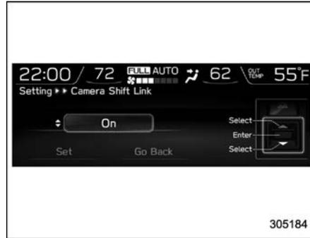
2. Select “On” or “Off” by using the control switches.
