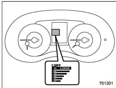
In the manual mode, you can use the center differential control switch to adjust the initial LSD torque as desired. When this mode is selected, the "AUTO" indicator disappears.
