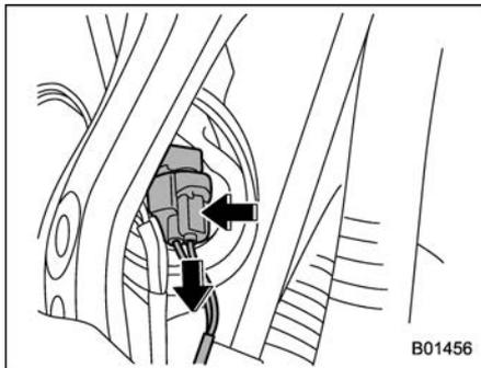
1. Disconnect the electrical connector from the bulb as pushing the tab.
