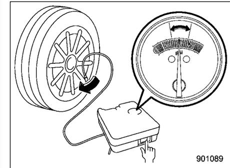
8. After driving for 10 minutes or 3 miles (5 km), whichever comes first, stop the vehicle in a safe place to recheck the air pressure (see step 4).
