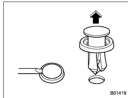
1. Pull out the center portion of the clip using a flat-head screwdriver as shown in the illustration.
