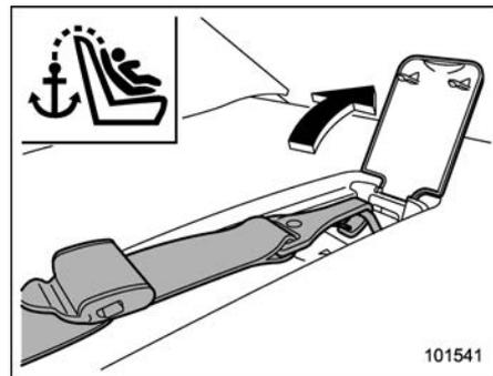
10. Latch the top tether hook onto the tether anchorage that is located behind the rear seat and tighten the top tether firmly. For additional instructions, refer to "Top tether anchorages" 1-33.
