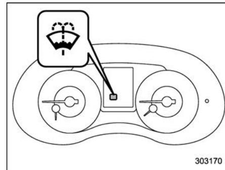
The windshield washer fluid warning indicator appears when the washer fluid level in the tank has dropped to the lower limit. If the warning indicator appears, refill the tank with fluid. For the refilling procedure, refer to “Windshield washer fluid”
