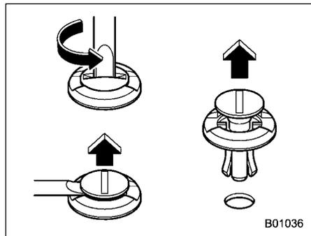
1. Turn the clips counterclockwise using a flat-head screwdriver until the center portion of the clip is raised.
