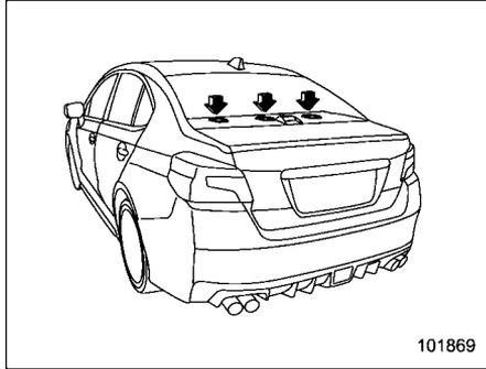
The tether anchorages (upper anchorages) are provided at the locations shown in the above illustration. For details, refer to “Top tether anchorages” ¶ 1-33.
