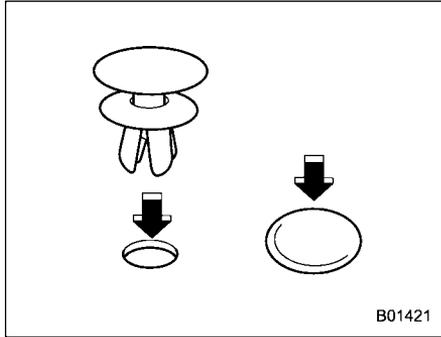
Insert the clip without the head first and then push the head of the clip into the hole.
