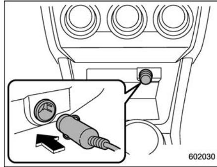
4. Connect the power plug of the air compressor into the accessory power outlet.
