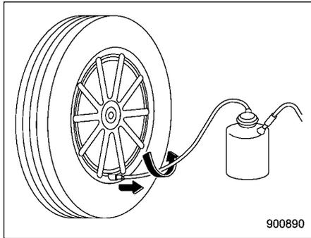
Remove the hose after filling the tire with air and fasten the valve cap.
