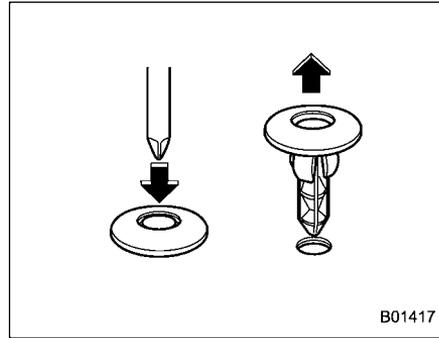
1. Push the center portion of the clip using a Phillips screwdriver until the clip is raised.
