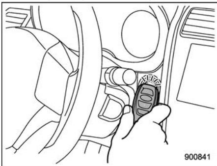
4. Hold the access key fob with the buttons facing you, and touch the push-button ignition switch with it.
