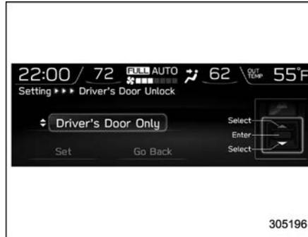
3. Select the preferred setting by using the control switches.
