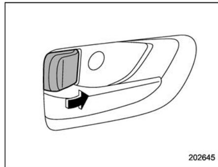
2. Rotate the lock lever forward.
