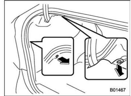
1. Remove the clips from the trunk trim with a flat-head screwdriver.
