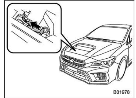
3. Release the secondary hood release by moving the lever between the front grille and the hood toward the left.
