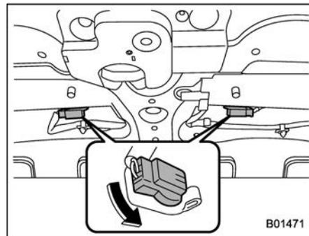
3. Turn the bulb socket counterclockwise and pull out the socket.
