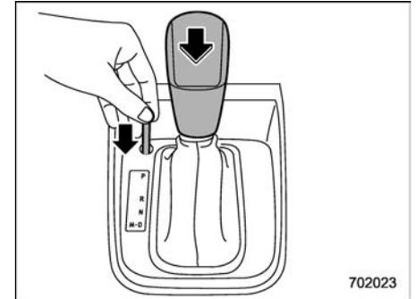
4. While depressing the brake pedal, insert a screwdriver into the hole, press the shift lock release button using a screwdriver, and then move the select
