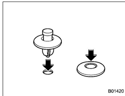
Insert the clip without the center portion first and then push the center portion of the clip into the hole.
