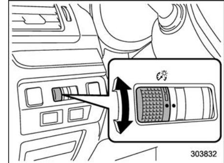
You can adjust the illumination brightness of the combination meter, the climate control panel, etc. by turning the control dial.
