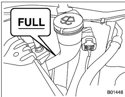
Remove the washer tank filler cap, then add windshield washer fluid until it reaches the "FULL" mark on the tank. If windshield washer fluid is unavailable use clean water.
