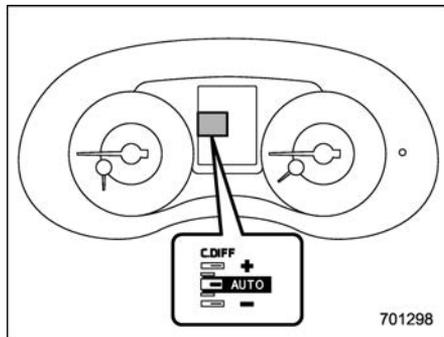
This indicator functions while the ignition switch is "ON". When it appears, it indicates that the driver's control center differential is set to the auto mode. It disappears when the driver's control center differential is set to the manual mode. For details, refer to "Driver's Control Center Differential (C.DIFF/DCCD) (STI)" 7-19.
