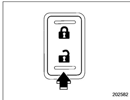
2. Hold down the REAR (UNLOCK) side of the power door locking switch.
