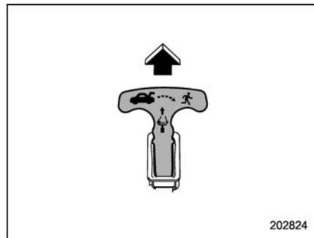
To open the trunk lid from inside the trunk, pull the yellow handle as indicated by the arrow on the handle. This operation unlocks the trunk lid. Then, push up the lid. The handle is made of material that remains luminescent for approximately an hour in the dark trunk space after it is exposed to ambient light even for a short time.
