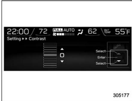
2. Select the contrast level by using the control switches.
