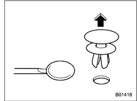
1. Pull out the head of the clip using a flat-head screwdriver as shown in the illustration.
