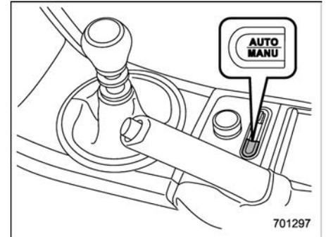
Press the "AUTO-MANU" switch on the center console to switch from auto mode to manual mode or vice versa. When you select the auto mode, the "AUTO" indicator appears. When you select the manual mode, the "AUTO" indicator disappears.
