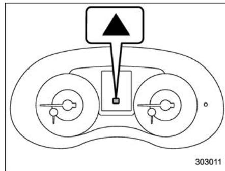
When the Intelligent (I) mode is selected, a shift-up indicator “▲” on the combination meter will blink to signal the best time to shift gears for maximum fuel efficiency.
