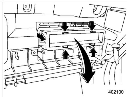
2. Remove the cabin air filter according to the following procedure in order to prevent dust on the air cleaner from falling to the inside of its housing.
