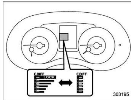
All the indicators will flash when the driver's control center differential has a malfunction. Have the vehicle inspected by your SUBARU dealer. For details, refer to "Driver's Control Center Differential (C.DIFF/DCCD) (STI)" 7-19.
