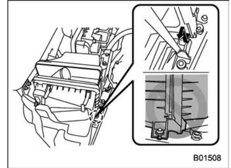
5. To install the air cleaner case cover, insert the projections on the air cleaner
