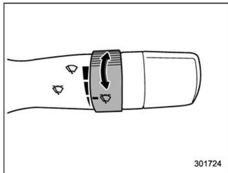
When the wiper switch is in the “
