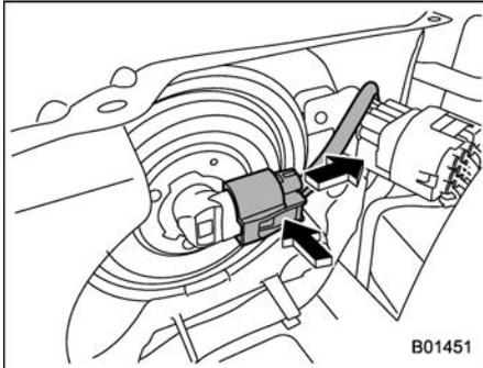
2. Disconnect the electrical connector from the bulb as pushing the tab.
