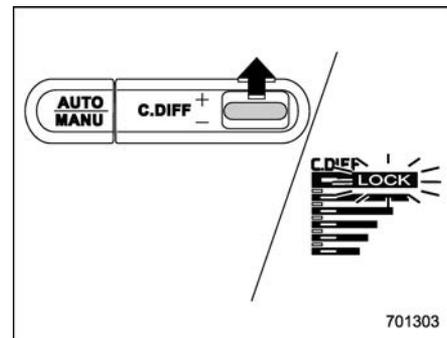
Push the switch forward to increase the initial LSD torque; when the "LOCK" indicator appears, the initial LSD torque setting is maximum. The center differential will then be almost completely locked.
