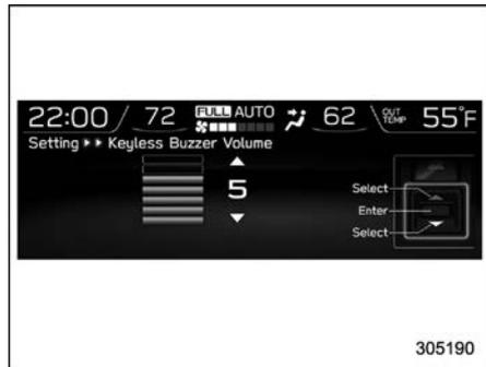
2. Select a volume level by using the control switches.
