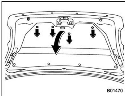
1. Open the trunk and remove the clips from the trunk lid trim with a flat-head screwdriver.
