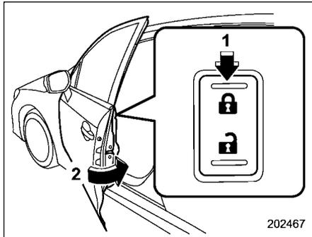
**Locking using power door locking switch**
