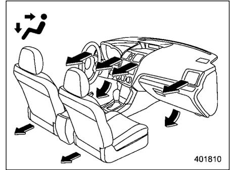
**(Bi-level):** Instrument panel outlets and foot outlets
