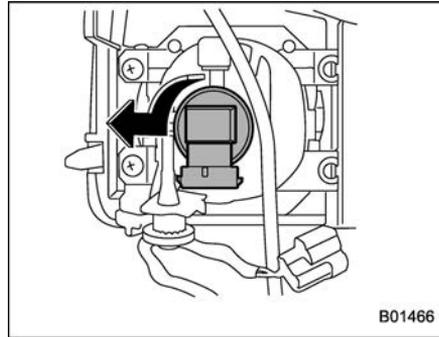
4. Remove the bulb by turning it counter-clockwise.
