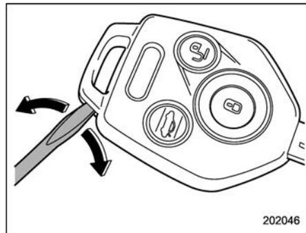
1. Open the key head using a flat-head screwdriver.
