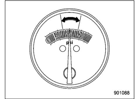
Apply the parking brake and turn on the ignition switch to the "ACC" position. Turn the air compressor switch on and adjust the air pressure to the appropriate level (green zone of the air gauge).
