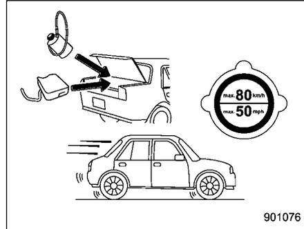
7. Stow the kit back in the vehicle and drive your vehicle immediately for 10 minutes or 3 miles (5 km).
