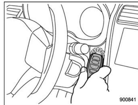
5. Hold the access key fob with the buttons facing you, and touch the push-button ignition switch with it.
