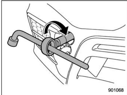
4. Tighten the towing hook securely using the wheel nut wrench.
