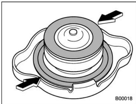
3. After refilling the reserve tank and the radiator, reinstall the cap and check that the rubber gaskets inside the radiator cap are in the proper position.
