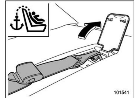
1. Open the cover and attach the top tether hook to the appropriate upper anchorage.
