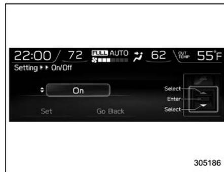
2. Select “On” or “Off” to turn the opening screen on or off by using the control switches.
