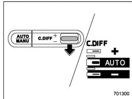
Pull the control switch rearward to select the "AUTO [-]" mode. After setting the mode, "AUTO [-]" appears.
