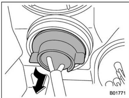
2. Remove the bulb from the headlight assembly by turning it counterclockwise.
