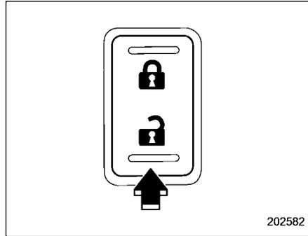
2. Push the rear side (unlock side) of the power door locking switch.
