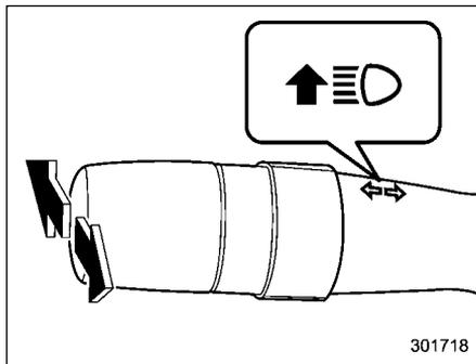
To change from low beam to high beam, push the turn signal lever forward. When the headlights are on high beam, the high beam indicator light “
