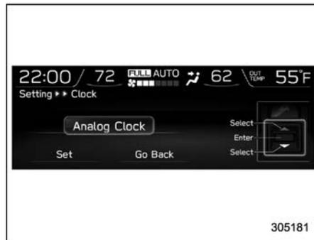
2. Select “Analog Clock”, “Calendar” or “Off” by using the control switches.
