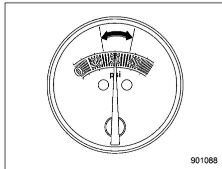
6. Turn the air compressor power switch off when the air pressure reaches the green zone of the air gauge. Remove the power plug from the accessory power socket.
