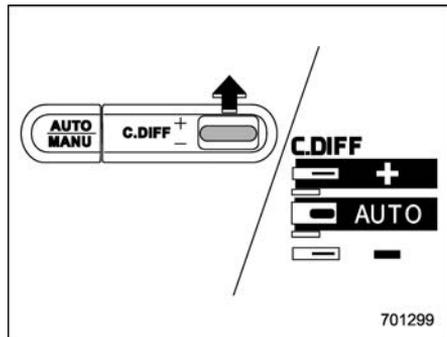
Push the control switch forward to select the "AUTO [+]" mode. After setting the
