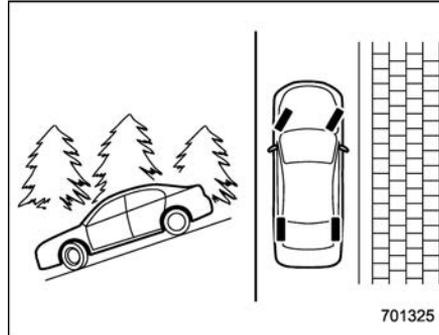
When facing downhill, turn the front wheels into the curb.
