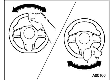
2. Use the cloth that was dampened with neutral detergent solution (5 - 10%) and strongly wrung out (A) and grip the steering wheel with it, then wipe by moving the cloth around the steering wheel as shown in the figure.
