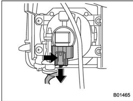
3. Disconnect the electrical connector from the bulb as pushing the tab.
