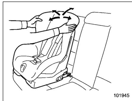
7. Before seating a child in the child restraint system, try to move it back and forth and right and left to verify that it is held securely in position.
