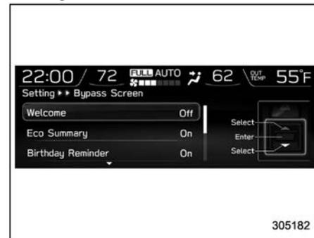
2. Select “On” or “Off” to turn the display of items on or off by using the control switches.
