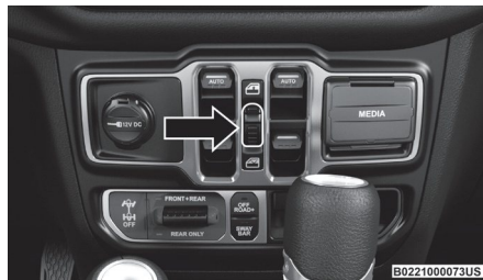
Window Lockout Switch
