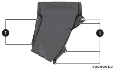
First Water Separation Chamber
