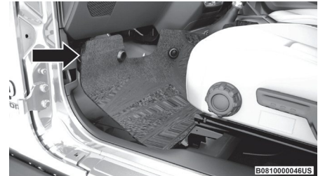
Front Carpet Pulled Away
