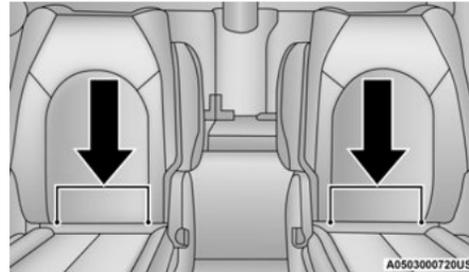
**LATCH Anchorages (Second Row Anchorages Shown)
