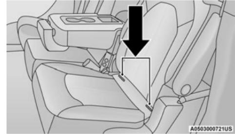
**LATCH Anchorages (Second Row Anchorages Shown)
