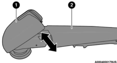
**Wiper Pivot Cap In Unlocked Position**
