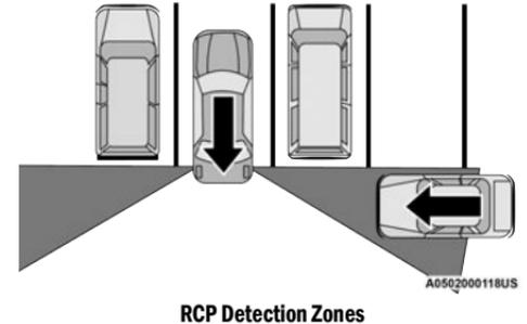
RCP monitors the rear detection zones on both sides of the vehicle, for objects that are moving toward the side of the vehicle with a minimum speed of approximately 3 mph (5 km/h), to objects moving a maximum of approximately 20 mph (32 km/h), such as in parking lot situations.
