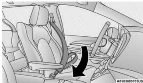
**Inserting Latch Plate Into Buckle**
