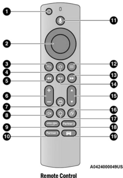
1. **Power Button** — Turns the screen for the selected channel on or off.
