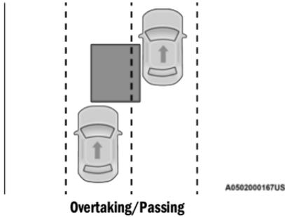
The BSM system is designed not to issue an alert on stationary objects such as guardrails, posts, walls, foliage, berms, snow banks, car washes, etc. However, occasionally the system may alert on such objects. This is normal operation and your vehicle does not require service.
