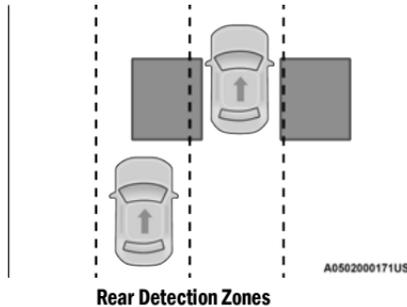
When the vehicle is started, the BSM Warning Light will momentarily illuminate in both outside rearview mirrors to let the driver know that the system is operational. The BSM system sensors operate when the vehicle is in any forward gear and enters standby mode when the vehicle is in PARK (P).
