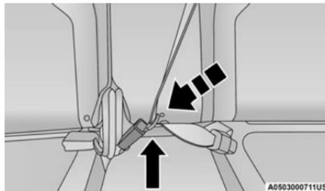
**Latch Plate And Buckle Connected**
