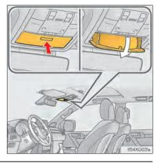
To use the overhead console when the conversation mirror is open, further extend the lid.  $(\rightarrow P.429)$
