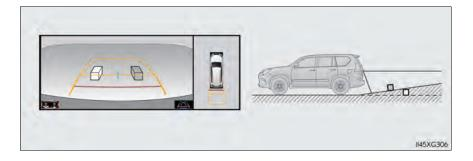
• When the ground behind the vehicle slopes down sharply The distance guide lines are displayed further away than the actual distance. Therefore, obstacles on a downward slope appear closer than the actually are. In the same way, the actual course of the vehicle will differ from the course indicated by the guide lines.
