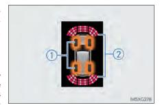
2 Pop-up display of the intuitive parking assist Displayed if an obstacle is detected while the intuitive parking assist is turned on.
