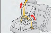
If the child restraint has a top tether strap, the top tether strap should be latched onto the top tether strap anchor.  $(\rightarrow P. 66)$
