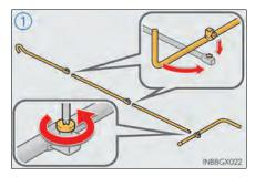
Assemble the jack handle extension bar and the jack handle bar and tighten the bolts.
