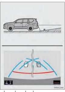
• When the ground behind the vehicle slopes down sharply
