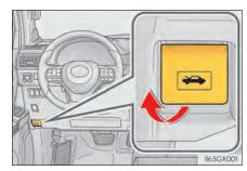
2 Move the auxiliary catch lever to side direction and lift the hood.
