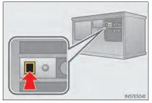
Press and hold the desired HomeLink<sup>®</sup> button (inside the vehicle) for 2 seconds and release it. Repeat this sequence (press/hold/release) up to 3 times to complete programming. If the garage door opener motor operates when the HomeLink<sup>®</sup> button is pressed, the garage door opener motor recognizes the HomeLink<sup>®</sup> signal.
