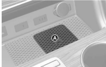
[A] Vehicle authentication pad (Wireless charging pad)
