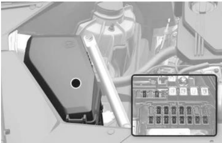
Cartridge type fuse
