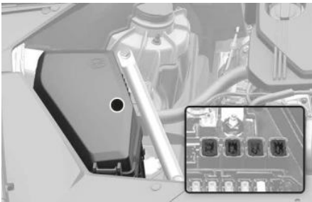
Cartridge type fuse
