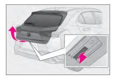
Raise the back door while pressing up the back door opener switch.
