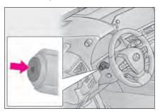
Press the Automatic High Beam switch.
