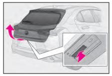
When the back door is unlocked: Press the back door opener switch.
