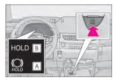
Turns the brake hold system on
