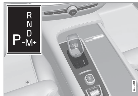
Overview of small gear selector and gear shift pattern in the instrument panel.
