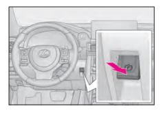
While the vehicle is stopped, press and hold the parking brake switch until "EPB Shift Interlock Function Activated" will be displayed on the multi-information display.
