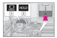
Turns the brake hold system on
