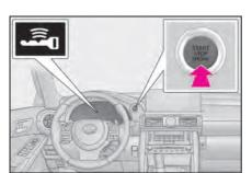
4 Press the engine switch shortly and firmly.
