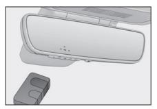
2 Point the remote control transmitter for the device at the rear view mirror, 1 to 3 in. (25 to 75 mm) from the HomeLink® buttons.
