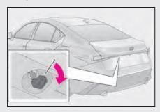
Turn the mechanical key clockwise to open.
