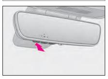
Press and hold the desired HomeLink<sup>®</sup> button (inside the vehicle) for 2 seconds and release it. Repeat this sequence (press/hold/release) up to 3 times to complete programming. If the garage door opener motor operates when the HomeLink<sup>®</sup> button is pressed, the garage door opener motor recognizes the HomeLink<sup>®</sup> signal.
