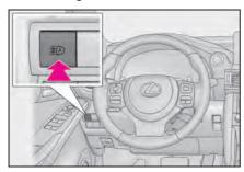
Press the Automatic High Beam switch.
