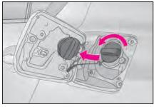
2 Turn the fuel tank cap slowly to remove it and put it into the holder on the fuel filler door.
