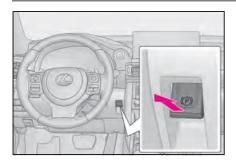
While the vehicle is stopped, pull and hold the parking brake switch until "EPB Shift Interlock Function Deactivated" will be displayed on the multi-information display.
