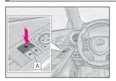
Press the switch to lock the passenger window switches.
