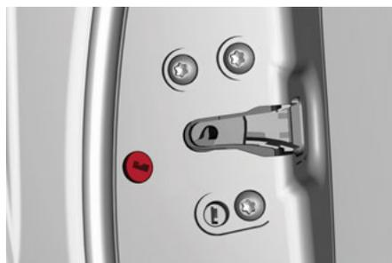
Door Lock Manual Release Lock Cylinder
