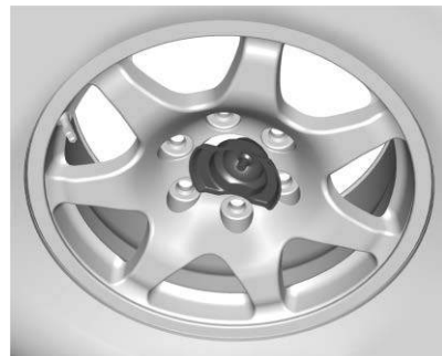
All Other Models Incorrectly Stored, Retainer Off-Center
