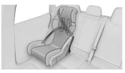
The seat belts in the rear and the front passenger seat belt can be permanently locked to fasten child restraint systems.
