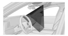
The camera in the headliner detects gestures that are carried out in the area of the center console at the height of the control display.
