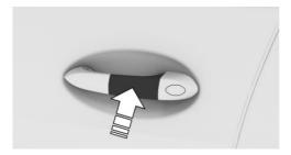
Hold the near field communication antenna of the smartphone directly and centered on the external door handle of the driver's door. The
