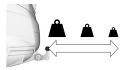
The permitted gross weight of the loaded rearmounted luggage rack depends on how far its center of gravity is from the ball head.
