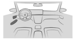
The central locking buttons are located on the front door.
