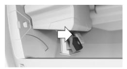
Slide the fragrance cartridge into the cartridge holder at a slight angle without applying pressure. The fragrance cartridge
