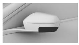
One exterior mirror camera is located at the bottom of each exterior mirror housing.
