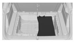
The cargo cover can be stowed under the cargo floor panel.
