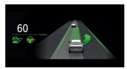
An example with active Driver Assistance: the indicator and warning lights for the distance control and the Automatic Lane Change Assistant indicate a lane change to the next lane. At the same time, the lane change to the next lane is shown with animation in the Assisted View.
