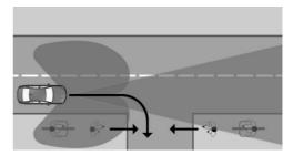
Sensors detect the traffic situation in their detection range when turning.
