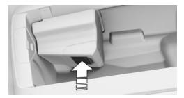
3. Remove the cover of the new fragrance cartridge. Hold the cover on the top to slide it from the fragrance cartridge.
