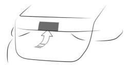
▶ Unlock the vehicle and then press the button on the trunk.
