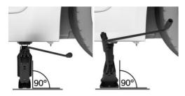
7. Crank the vehicle up until the vehicle jack has the entire surface on the ground and the relevant wheel is maximum 1.2 inches/3 cm above ground.
