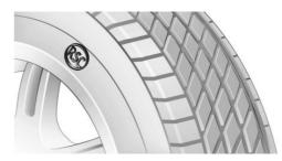
Runflat tires are labeled with a circular icon containing the letters RSC marked on the tire sidewall.
