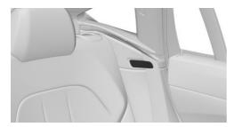
2. Pull the lever and fold the rear seat backrest forward.
