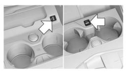
A USB port is located in the center console at one of the marked positions.
