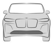
The front radar sensor is located in the front bumper.
