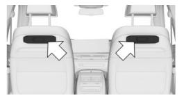
The mounts and USB ports are located behind the marked covers.
