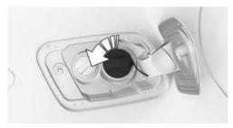
3. Place the fuel filler cap in the mount on the fuel filler flap.
