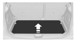
To open the storage compartment, pull the cargo area floor upward using the loop and fold it open.
