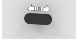
To adjust the seat in the longitudinal direction, press the longitudinal direction switch forward or backward.
