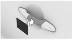
To unlock/lock the vehicle using the Key Card, hold the activated Key Card directly over the middle of the driver's door handle.
