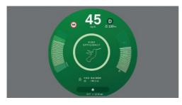
The efficient range of the power gauge is colored green. Additionally, the bonus range will be displayed.
