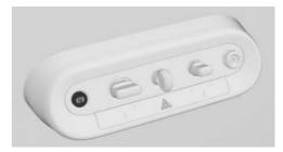
To engage selector lever position P and the parking brake, press the parking brake button on the switch cluster.
