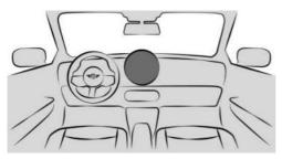
The Interaction Unit is located on the instrument panel above the center console.
