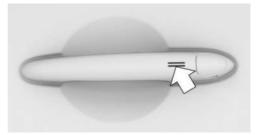
To close a window using the door handle, touch the grooved surface on the closed driver's door handle with your finger and hold it there without gripping the door handle.
