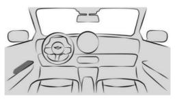
The central locking system buttons are located on the driver's door.
