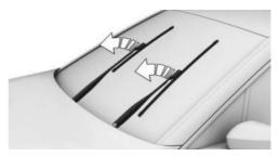
3. Press the button on the wiper, arrow 1, turn the wiper blade clockwise slightly, then pull it forward and out, arrow 2.
