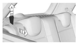
On the rear seat backrest, pull the loop, arrow 1, and fold the rear seat backrest forward, arrow 2.
