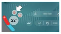
2. Press the steering wheel heating button repeatedly until the desired level is selected, arrow.
