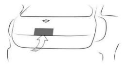
To access the vehicle while it is in deep sleep mode, press the Open button in the cargo area. Deep sleep mode remains on in this case.
