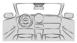
The interior camera is located in the headliner.
