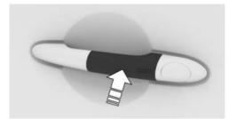
To unlock/lock the vehicle with the MINI Digital Key, hold the smartphone's NFC antenna directly over the middle of the driver's door handle. The position of the near field communication antenna depends on the smartphone model.
