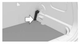
Insert the cargo area floor from above into the lower position of the holder, then fold it down.
