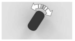
To adjust the backrest tilt, flip the backrest tilt switch forward or backward.
