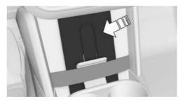
1. To turn on drive-ready state with the MINI Digital Key, place the smartphone in the center of the tray on the center console and slide it down behind the holder.
