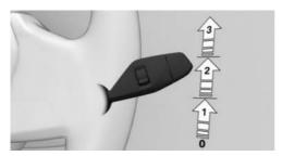
To activate the rain sensor: Push the wiper lever upward from position 0, arrow 1, once. To deactivate the rain sensor: Push the wiper lever back to position 0.
