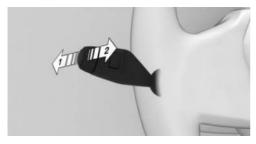
Press the turn signal lever forward, arrow 1, or pull the turn signal lever backward when the high-beam headlights are on, arrow 2.
