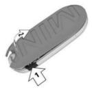
2. Pull the cover out of the upper locking mechanism, arrow, then remove the cover.
