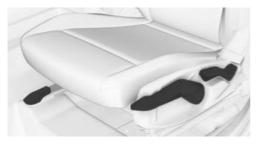
The levers for setting the seats are located on the front seats.
