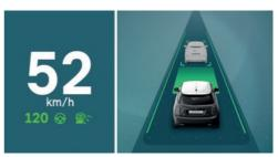
An example of active Driver Assistance: Indicator lights and warning lights for Distance Control and Assisted Driving Mode are displayed. At the same time, the Distance Control is animated in Assisted View.
