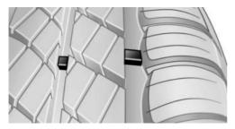
The tire manufacturer's wear indicators are distributed over the tire circumference. These indicators have a height of min.
