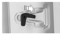
2. Pull and hold the driver's door handle outward with one hand.
