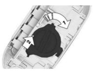
7. Insert the cover in reverse order, arrow 1 and arrow 2. The cover must audibly engage at the top and bottom.
