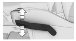
To adjust the height: On the side of the seat, push the seat height lever up or down as many times as necessary for the seat to reach the desired height.
