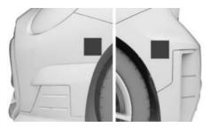
The ultrasonic sensors for the parking assistance systems are located on the sides of the front and rear bumpers.
