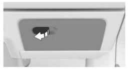
Pull the handle on the glove compartment.
