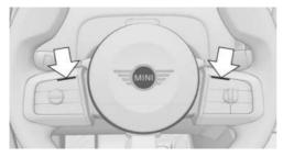
Similar to the displays for Assisted Driving Mode on the Interaction Unit, the two LEDs above the keypads on the steering wheel illuminate.
