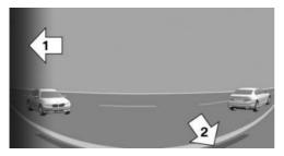
The respective boundary area, arrow 1, in the camera image flashes red if vehicles are detected by the sensors.
