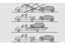
The vehicle should be transported with a tow truck with a so-called spectacle lift or on a loading platform.
