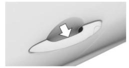
To unlock the vehicle using the door handle, reach into the recessed grip on the driver's door.
