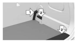
Insert the cargo area floor into the upper position of the holder, arrow 1, then place it on the console and edge of the rear wall, arrow 2.
