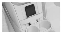
Insert the smartphone upright and in the center, behind the holder, and slide it down to the stop. The smartphone display must point upward.
