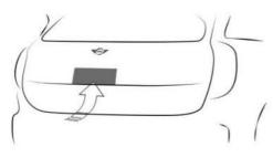
Unlock the vehicle, then press the unlock button on the outside of the trunk. Swivel the tailgate upward.
