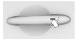
To close the glass sunroof using the driver's door handle, touch the grooved surface on the driver's door handle with your finger and hold it there without reaching into the recessed grip.
