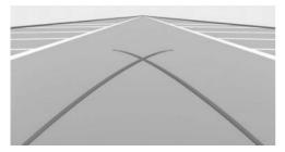
The Interaction Unit camera view includes turning circle lines that show the path with the smallest possible turning circle on a level road.
