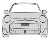
The front camera is located above the license-plate carrier.
