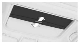
To open/close the sun protection, slide the sun protection to the desired position using the handle.
