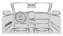
The power window switches are located on the doors.
