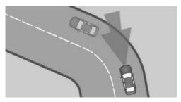
When Distance Control is on, if your set speed is too high for a bend, your vehicle will be slowed slightly in the bend. Because curves may not be anticipated in advance, drive into a curve at an appropriate speed.
