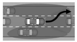
The sensors monitor and detect the clearance in front of the vehicle. Depending on the vehicle equipment, the areas next to the vehicle are also monitored.
