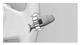
To adjust the sensitivity of the rain sensor, turn the knurled wheel on the wiper lever as follows:
