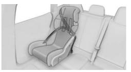
The seat belts in the rear and the front passenger seat belt can be permanently locked to fasten child restraint systems.
