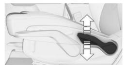
To adjust the backrest tilt, pull the backrest tilt lever on the side of the seat and tighten or loosen the backrest as required.
