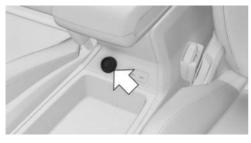
A socket is provided on the center console under a cover. Pull off the cover before using the socket.
