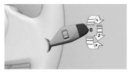
To turn on the rear wiper, rotate the outer switch on the wiper lever upward.
