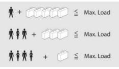
The maximum payload is the sum of the weight of the occupants and the cargo.
