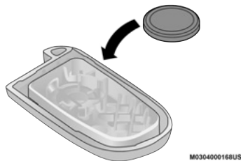
Key Fob Battery Replacement
