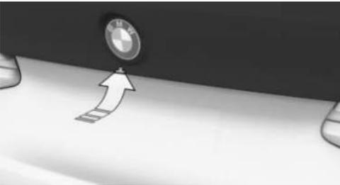
Press the button on the outer side of the trunk lid.
