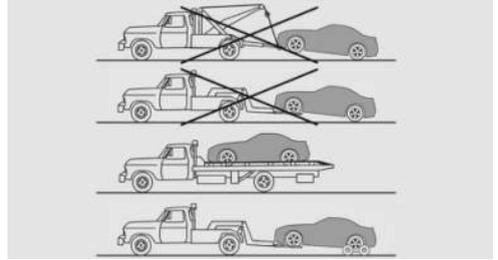
Have vehicle transported on a loading platform or use a tow dolly.
