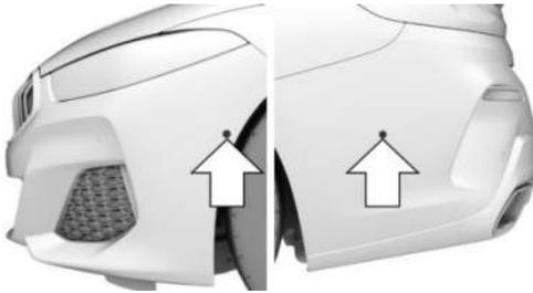
The ultrasonic sensors for Parking Assistant are located to the side in the front and rear bumpers.
