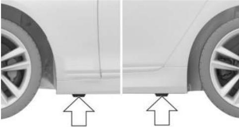
The jacking points are located at the indicated positions.
