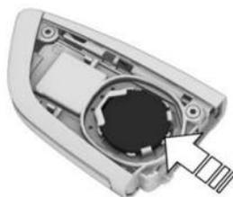
4. Insert a type CR 2032 3 V battery with the positive side facing up.
