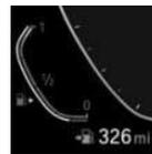
An arrow next to the fuel pump icon indicates the vehicle side on which the fuel filler flap is located.
