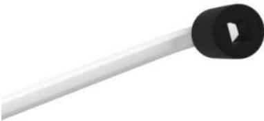
4. Position the hexagon wrench with inserted adapter on the convertible top locking (arrow).
