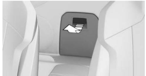
3. In the cargo area: open flap completely. The flap is secured with a magnet.
