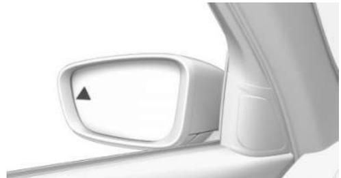
The warning light in the exterior mirror warns of a possible collision with a detected vehicle.
