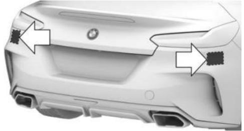
The radar sensors are located to the side behind the rear bumper.
