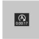
ECO PRO driving mode: depending on the vehicle equipment, the total time that the engine has been switched off using the Auto Start/Stop function is displayed on an automatic engine stop.
