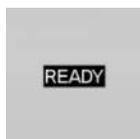
READY is displayed in the instrument cluster. The Auto Start/Stop function is ready for automatic engine start.
