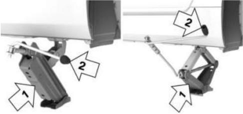
2. Insert the jack into the rectangular recess of the jacking point closest to the wheel to be changed.
