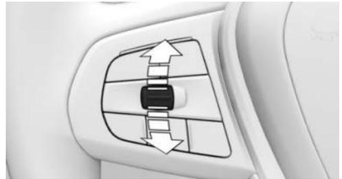
Press the rocker switch up or down once while the system is interrupted. The system will be activated.
