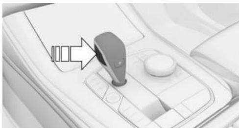
Press and hold the button to release the selector lever lock.
