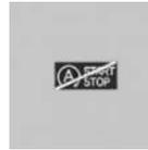
The display indicates that the conditions for an automatic engine stop have not been met.
