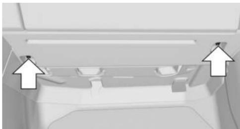
Loosen fasteners, arrows, and open cover.
