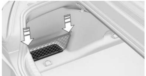
Smaller items can be stowed behind the net on the left side. To transport larger objects, slide the net down. Grab the top of the net as close as possible to the edge next to the holder. At first, a resistance must be overcome.
