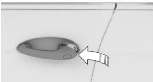
2. Guide one finger of your other hand from the back under the cover cap and push the cover cap out.
