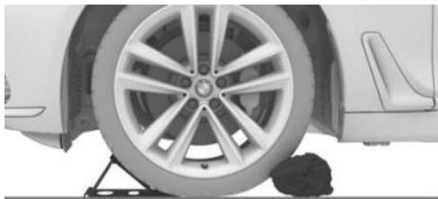
Place chocks or other suitable objects in front and behind the wheel that is diagonal to the wheel being changed.
