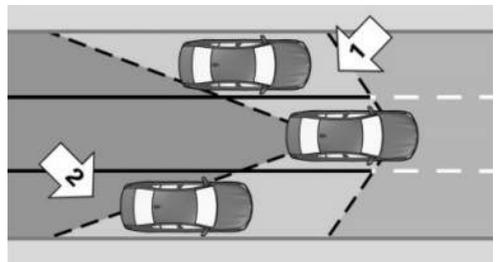
Radar sensors monitor the area behind and next to the vehicle when traveling faster than a minimum speed.
