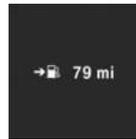
The current range is displayed as numerical value between speedometer and tachometer.
