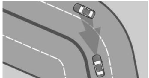
When you approach a curve the system may briefly report vehicles in the next lane due to the bend of the curve. If the system decelerates you may compensate for it by briefly accelerating. After releasing the accelerator pedal the system is reactivated and controls speed independently.
