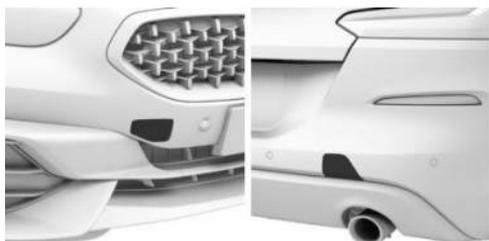
Press on the mark on the edge of the cover to push it out.
