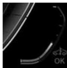
▶ Cold engine: the needle is at the low temperature value. Drive at moderate RPM and vehicle speeds.
