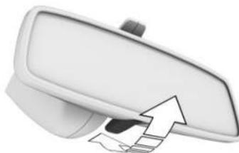
To reduce the blinding glare of the interior mirror, flip the lever forward.
