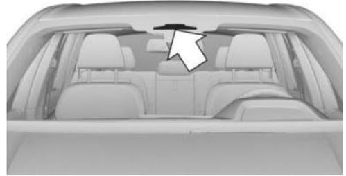
The cameras behind the windshield are located near the interior mirror.
