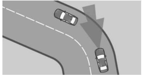
When the set speed is too high for a curve, the speed is reduced slightly. Because curves may not be anticipated in advance, drive into a curve at an appropriate speed.
