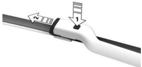
4. Insert the new wiper blade and press it on until it you hear it snap into the holder.
