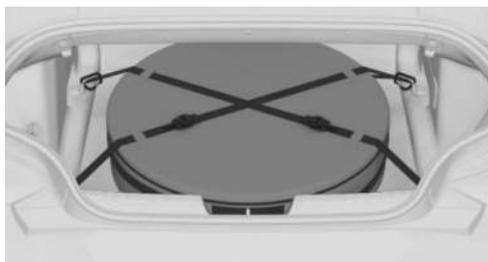
The emergency wheel and wheel change tools are located in a bag in the cargo area.
