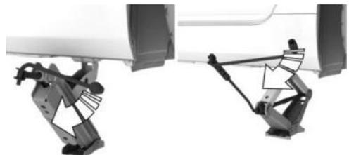
4. Take your hand away from the jack as soon as the jack is under load and continue turning the jack crank handle or lever with one hand.
