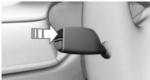
Continue to press the button on the turn signal lever until the desired widget is selected.
