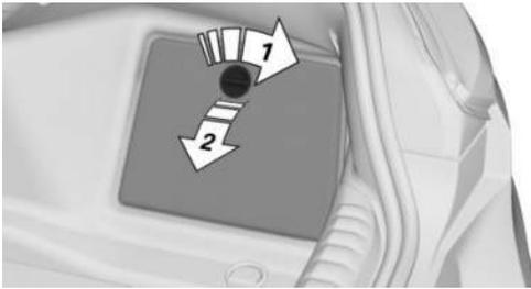
The onboard vehicle tool kit is located under a cover on the right side of the cargo area.
