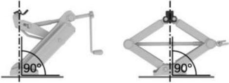
6. Crank the vehicle up until the vehicle jack has the entire surface on the ground and the relevant wheel is maximum 1.2 inches/3 cm above ground.
