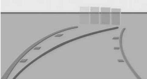
Depending on the equipment, obstacles behind the vehicle are detected by the Park Distance Control sensors.
