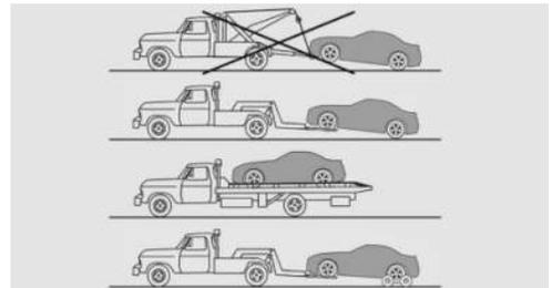
Have the vehicle transported by a tow truck with spectacle lift, on a loading platform, or with a tow dolly.
