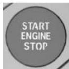
Pressing the Start/Stop button switches drive-ready state on or off.
