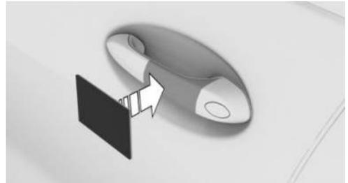
Hold the activated Key Card directly at the center of the driver's door handle.
