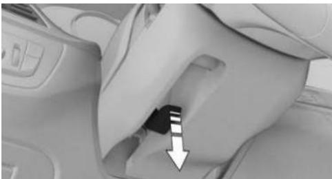
1. Fold the lever down completely.
