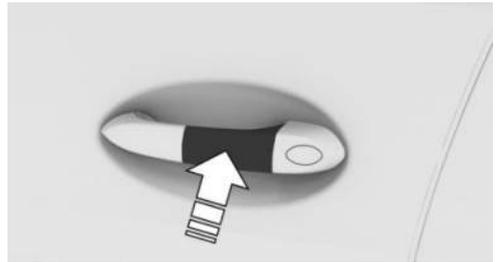
Hold the smartphone NFC antenna directly at the center of the driver's door handle.
