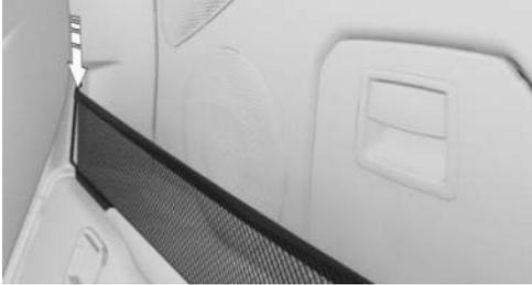
Slide the upper edge of the net up to the correct height. Grab the top of the net as close as possible to the edge next to the holder. At first, a resistance must be overcome.
