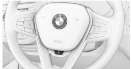
Button for steering wheel heating
