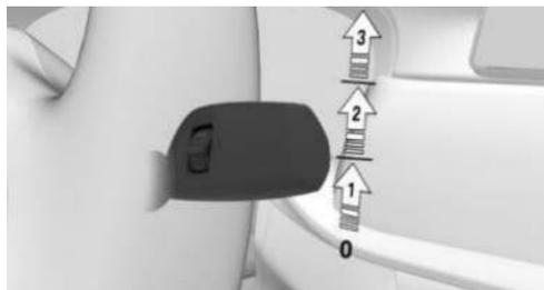
Activate: press the lever up once from its 0 position, arrow 1.
