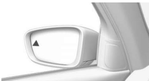
The warning light in the exterior mirror flashes if the rear sensors detect other vehicles when the vehicle is reversing.
