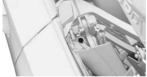
4. Lift the convertible top out on the front on both sides, and swing it forward.
