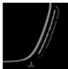
▶ Cold engine: the LEDs of the indicator show a low temperature value. Drive at moderate RPM and vehicle speeds.
