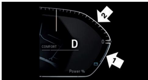
Needle in the area of arrow 1: display of the energy recovered by coasting or when decelerating, CHARGE.
