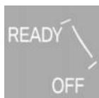
The word OFF in the tachometer indicates that drive-ready state is switched off and standby state is switched on.
