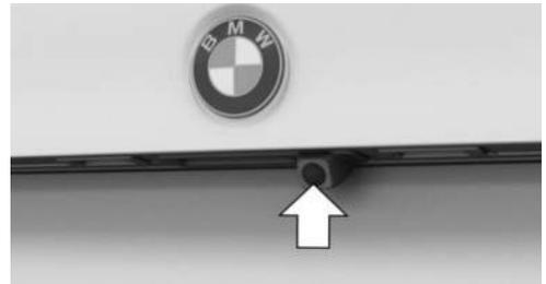
The Rear View Camera is located in the trunk lid handle.
