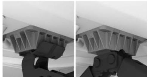
3. Extend the jack by turning the jack crank handle or lever clockwise.
