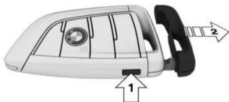
Press the button, arrow 1, and pull out the integrated key, arrow 2.
