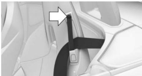
When buckling seat belts, make sure the seat belt guide is closed.
