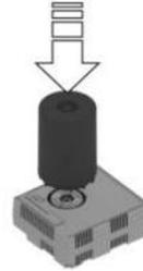
2. Turn the sealant bottle clockwise by 90° to the stop.
