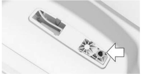
5. While one person presses the center of the front convertible top frame from the outside onto the windshield frame: turn the hexagon wrench counterclockwise to the stop to close the locking hooks. The front convertible top frame must be locked in the windshield frame.
