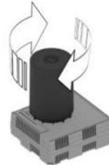
3. Connect the filler hose to the outlet of the sealant bottle and turn clockwise by 90° to the stop.
