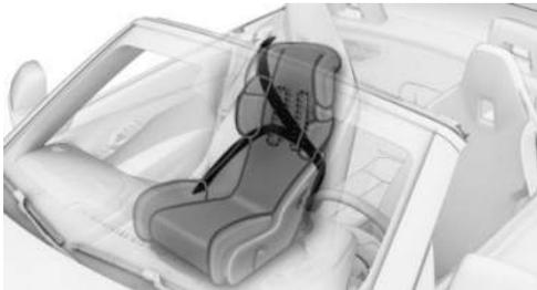
The seat belt on the passenger's side can be locked to fasten child restraint systems.
