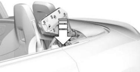
3. Turn the screw on the left side of the vehicle counterclockwise to the stop. Turn the
