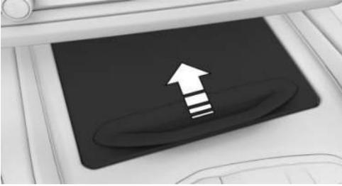
2. The socket is located next to the wireless charging tray. Detach the cover.
