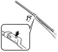
3. Pull the blade rubber in the direction of the arrow and slide it to a position where the blade holder groove can be checked.
