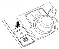
If the EPB switch is pressed without depressing the brake pedal, the display or indicator light in the instrument cluster notifies the driver that the brake is not depressed.
