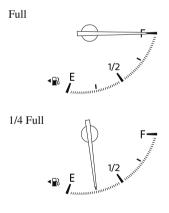
If the low fuel warning light illuminates or the fuel level is very low, refuel as soon as possible.
