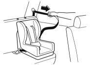
6. Push the child-restraint system firmly into the vehicle seat. Be sure the belt retracts as snugly as possible. A clicking noise from the retractor will be heard during retraction if the system is in the automatic locking mode. If the belt does not lock the seat down tight, repeat this step.
