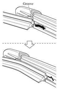
6. After pulling the blade rubber in the direction of the arrow and sliding the blade rubber to a position to check the
