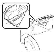
If it is at or near L, add enough coolant to the coolant reservoir to provide freezing and corrosion protection and to bring the level to F.
