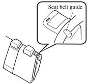
2. Press the seatback rearward and lock it in place. After returning the seatback to its upright position, make sure it is securely locked.
