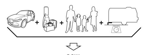
**GCW (Gross Combination Weight)** is the weight of the loaded vehicle (GVW) plus the weight of the fully loaded trailer.
