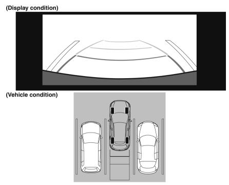
6. When the selector lever is shifted from reverse (R) position to another selector lever position, the screen returns to the previous display.
