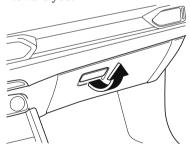
To close the glove compartment, firmly press in the center of the glove compartment lid.
