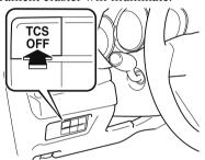
Press the switch again to turn the TCS back on. The TCS OFF indicator light will turn off.
