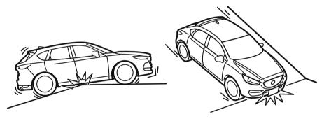
This vehicle is equipped with low profile tires allowing class-leading performance and handling. As a result, the sidewall of the tires are very thin and the tires and wheels can be damaged if driven through potholes or on rough/uneven roads at excessive speeds. Use care and reduce speed when traveling on rough/uneven roads or through potholes.
