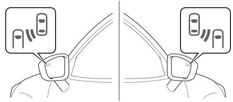
When the ignition is switched ON, the warning indicator light turns on momentarily and then turns off after a few seconds
