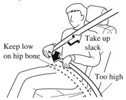
Before fastening the rear seat belt, make sure that the seat belt passes through the seat belt guide correctly and it is not twisted
