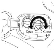
Remove the cap of a bottle containing DEF, insert the bottle into the DEF filler port, and screw it in lightly until it stops.
