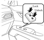
To lock all the doors and the liftgate from an open front door, press the lock side of the door lock switch and then close the door.
