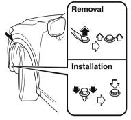
4. Pull the center of each plastic retainer using a flathead screwdriver and remove the retainers, and then partially peel back the mudguard.
