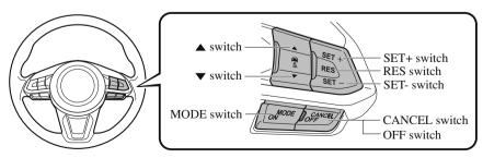
When the MODE switch is pressed once, the MRCC with Stop & Go function system turns on, and the MRCC with Stop & Go function main indication (white) turns on and the vehicle speed and the distance between the vehicles while in headway control can be set.
