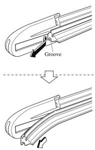
5. Insert the end of the new blade rubber into the groove of the blade holder
