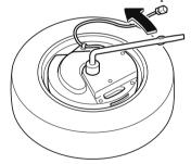
For vehicles not equipped with a sub-woofer, turn the spare tire
