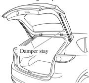
➤ Do not modify or replace the liftgate damper stay. Consult an Authorized Mazda Dealer if a liftgate damper stay is deformed or damaged for reasons such as a collision or if there is some other problem.
