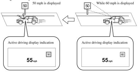
The excessive speed warning is initially set to inoperable. If you want to activate the excessive speed warning, change the setting in the personalization features. In addition, the warning pattern and the warning activation timing differ depending on the setting contents. Refer to the Settings section in the Mazda Connect Owner's Manual.
