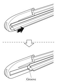
4. Pull the end of the blade rubber from the blade holder groove in the direction
