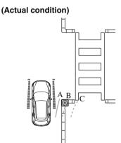
Make sure that there are no obstructions within the projected vehicle path lines. Turn the steering wheel so that the projected vehicle path lines travel inside of the obstruction (A), and drive the vehicle forward until it passes the obstruction. If the projected vehicle path lines are on an obstruction (B) or outside of the obstruction (C), the vehicle may contact the obstruction when turning the vehicle sharply.
