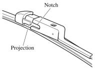
10. Slide the blade component and install it to the wiper arm.
