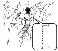
The top of the float should be between F and L.
