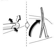
Firmly rotate the wiper blade to the right until it unlocks, then remove the blade.
