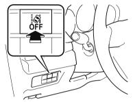
Drive the vehicle in the center of the driving lane while the LAS & LDWS OFF indicator light in the instrument cluster is turned off.
