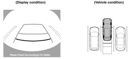
6. When the selector lever is shifted from R to another selector lever position, the screen returns to the previous display.
