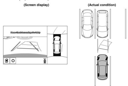
Make sure that there are no obstructions within the projected vehicle path lines. Drive the vehicle forward while turning the steering wheel so that no obstructions come within the projected vehicle path lines.
