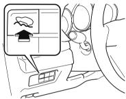
If the switch is pressed again, the Off-Road Traction Assist is stopped and the Off-Road Traction Assist indicator light turn off.
