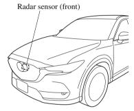
If "Front Radar Sensor Blocked" is displayed in the multi-information display of the instrument cluster, clean the area around the radar sensor (front).
