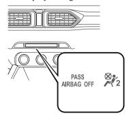
If the front passenger occupant classification sensor is normal, the indicator light turns on when the ignition is switched ON. The light turns off after a few seconds. Then, the indicator light turns on or is off under the following conditions:
