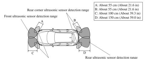
Front corner ultrasonic sensor detection range
