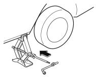
7. Turn the jack handle clockwise and raise the vehicle high enough so that the spare tire can be installed. Before removing the lug nuts, make sure your
