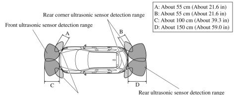
Front corner ultrasonic sensor detection range
