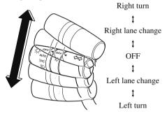
The turn signal indicators in the instrument cluster flash according to the operation of the turn signal lever to show which signal is working.
