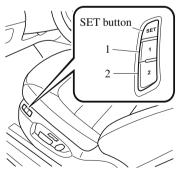
A driving position can be programmed or operated using the buttons on the side of the seat or the key.
