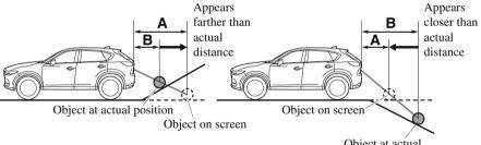
A: Distance between the vehicle and object displayed on the screen.
