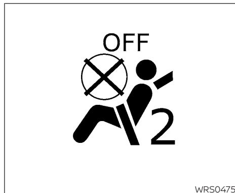
Front passenger air bag and status light
