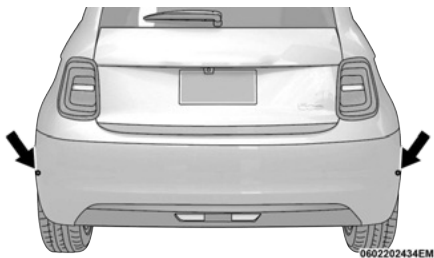
Radar Sensors Location
