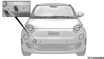
Front Tow Hook Installed
