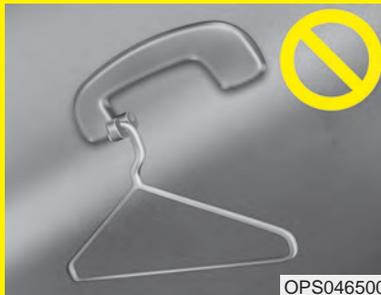
**Do not hang other objects such as hangers or hard objects except clothes. Also, do not put heavy, sharp or breakable objects in the clothing's pockets. In an accident or when the curtain air bag is inflated, it may cause vehicle damage or personal injury.**
