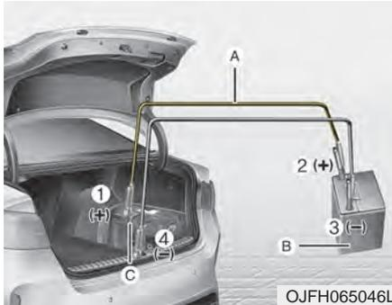
Connect cables in numerical order and disconnect in reverse order.
