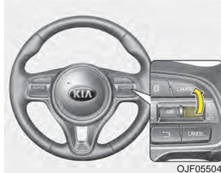
If any method other than the CRUISE ON-OFF switch was used to cancel cruising speed and the system is still activated, the most recent set speed will automatically resume when you move the lever up.
