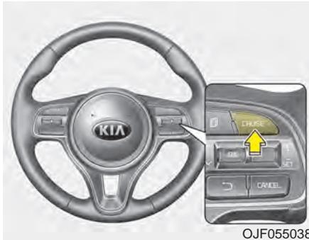
1. Press the CRUISE button on the steering wheel to turn the system on. The CRUISE indicator light in the instrument cluster will illuminate.
