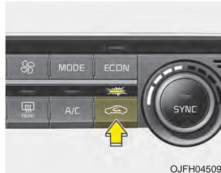
This is used to select the outside (fresh) air position or recirculated air position.
