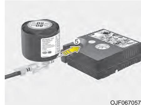
7. Insert the sealant bottle into the housing (5) of the compressor so that the bottle is upright.
