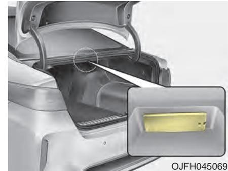
If the trunk lamp (LED) (1) does not operate, have the vehicle checked by an authorized Kia dealer.
