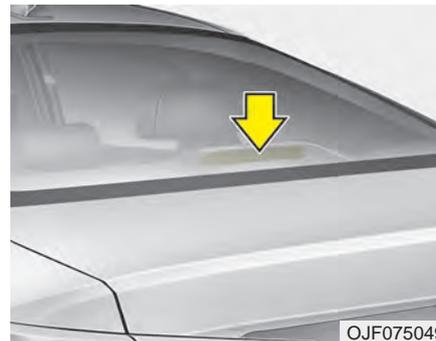
If the high mounted stop lamp (LED) does not operate, have the vehicle checked by an authorized Kia dealer. The LED lamps cannot be replaced as a single component because they are part of an integrated unit. The LED lamps have to be replaced with the unit. A skilled technician should check or repair the high mounted stop lamp (LED), to avoid damage to related parts of the vehicle.
