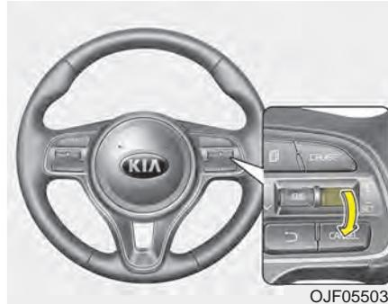
3. Move the lever down (to SET-), and release it at the desired speed. The SET indicator light in the instrument cluster will illuminate. Release the accelerator at the same time. The desired speed will automatically be maintained.
