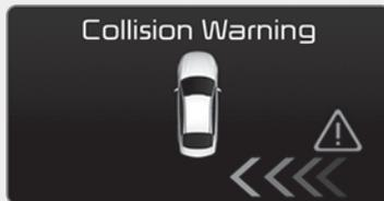
If the vehicle detected by the sensors approaches your vehicle, the warning chime will sound, the warning light on the outside rearview mirror will blink and a message will appear on the LCD display.
