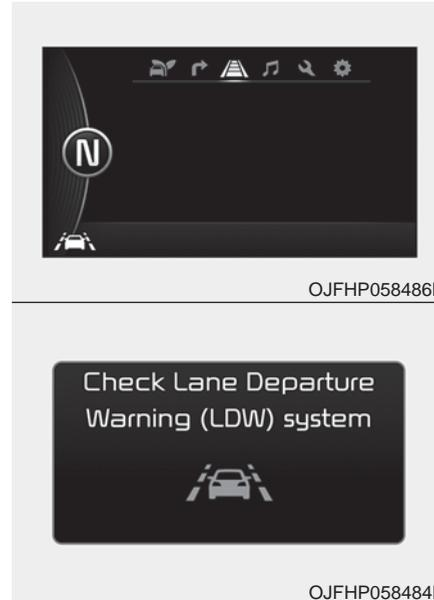
When the LDW is not working properly, the warning light will illuminate and the warning message will come on for a few second. After the message disappears, the master warning light will illuminate.
