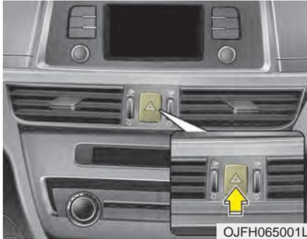
Depress the flasher switch with the ignition switch in any position. The flasher switch is located in the center fascia panel. All turn signal lights will flash simultaneously.
