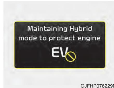
The engine will automatically stop after sufficient heating. If the engine is turned OFF without sufficient heating, the engine maintenance mode will be operated once more.
