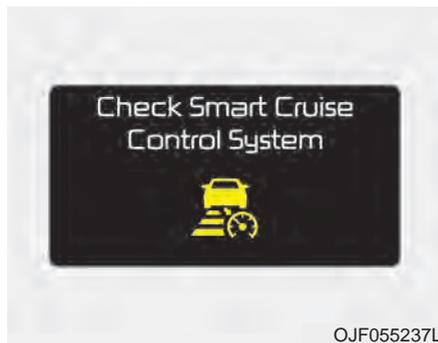
The message will appear when the vehicle to vehicle distance control system is not functioning normally. In this case, take your vehicle to an authorized Kia dealer and have the system checked.
