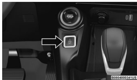
Stop/Start OFF Switch
