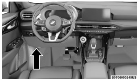
Interior Fuse Box Location
