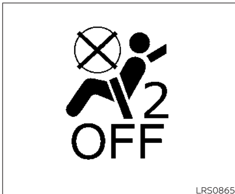
Front passenger air bag and status light
