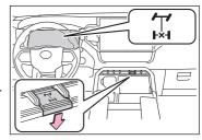
To unlock the rear differential, push the switch again.
