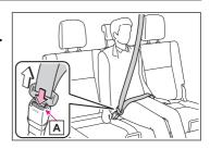
2 Insert the mechanical key (→ P.126) or plate B into the notch of buckle and remove the belt.
