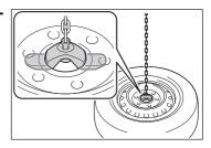
4 While raising, secure the tire, taking care that the tire goes straight up without catching on any surrounding part, to prevent it from flying forward during a collision or sudden braking.
