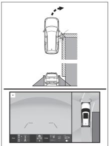
The pillar that is diagonal to the parking spot may be displayed perpendicular on the screen. Even if it seems like there will not be a collision, the pillar is diagonal, so there may be collision with the upper part of the pillar.
