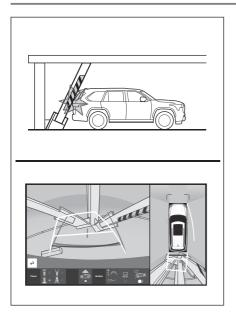
Visually check the surroundings and the area behind the vehicle. In the case shown below, the truck appears to be outside of the estimated course lines and the vehicle does not look as if it hits the truck. However, the rear body of the truck may actually cross over the estimated course lines. In reality if you back up as guided by the estimated course lines, the vehicle may hit the truck.
