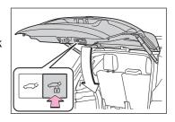
Also, if the power back door enters the sensor area during the closing process, the power back door will stop.
