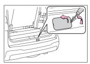
3 Insert the end of the jack handle extension into the lowering screw and turn it counterclockwise.
