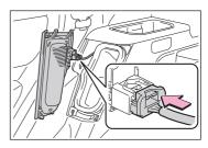
9 Install the air intake vent cover.
