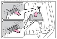
▶ Engine compartment: type B fuse box
