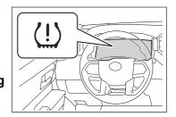
Afterward, the tire pressure warning light turns on after flashing for 1 minute.
