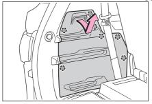
Remove the positive (+) battery terminal cover.
