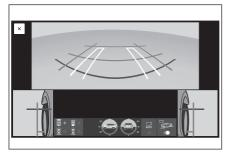
When the front view and side view screens are touched, each of the display sizes can be changed.
