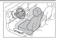
When all of the following have been performed, the driver's seat and steering wheel (power adjustment type) are automatically adjusted to a position that allows driver to enter and exit the vehicle easily.
