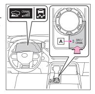
2 Turn the mode select switch left or right to select a mode on the multi-information display.
