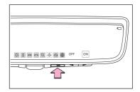
2 Press [ ] or [ ] to enable ([ON])/disable ([OFF]) the automatic antiglare function.
