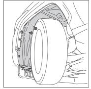
2 Open the fender liner and turn the bulb base counterclockwise.
