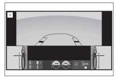
When the under vehicle terrain view and side view screens are touched, each of the display sizes can be changed.
