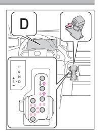
[ ]: While the power switch is in ON and the brake pedal depressed\*1, shift the shift lever while pushing the shift release button on the shift knob.
