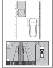
Check the positions and distance between the vehicle width guide line and a target object such as the obstacle or curb of the road.
