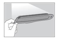
7 Reinstall the filter to the cover.
