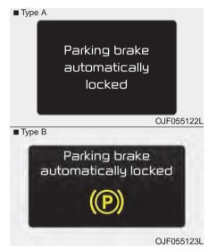
Parking brake automatically locked When the EPB is applied from Auto Hold, a warning will sound and a message will appear.
