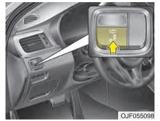
The indicator on the switch will illuminate when the Blind Spot Detection System (BSD) switch is pressed with the Engine Start/Stop Button ON.
