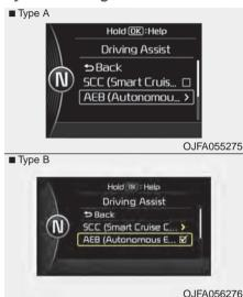
The driver can activate the AEB by placing the ignition switch to the ON position and by selecting 'User Settings', 'Driving Assist', and 'Autonomous Braking System'. The AEB deactivates, when the driver cancels the system setting.
