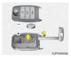
A smart key battery should last for several years, but if the smart key is not working properly, try replacing the battery with a new one. If you are unsure how to use your smart key or replace the battery, contact an authorized Kia dealer.
