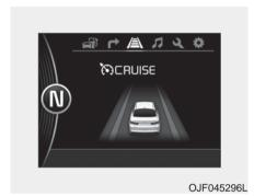
This mode displays the state of the Advanced Smart Cruise Control (ASCC) and Lane Departure Warning System (LDWS).
