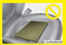
not place electronic devices such as laptops, DVD player, or conductive materials such as water bottles on the passenger seat.
