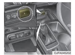
A wireless smart phone charging system located in front of the center console
