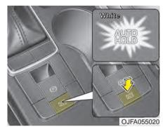
1.Depress the brake pedal, start the engine and then press the Auto Hold button. The white AUTO HOLD indicator will come on indicating the system is in standby. Before the Auto Hold will engage, the driver's door, engine hood must
