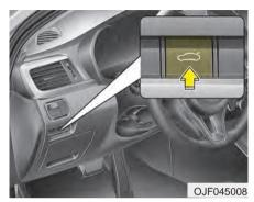
To open the trunk from inside the vehicle, push the trunk lid release button.
