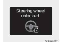
• This warning message illuminates if the steering wheel does not lock when the Engine Start/Stop Button changes to the OFF position.
