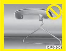
Do not hang other objects such as hangers or hard objects except clothes. Also, do not put heavy, sharp or breakable objects in the cloth pockets. In an accident or when the curtain air bag is inflated, it may cause vehicle damage or personal injury.
