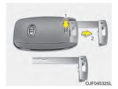
To remove the mechanical key, press and hold the release button(1) and remove the mechanical key (2).
