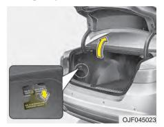
If the fuel filler lid does not open using the remote fuel filler lid release, you can open it manually. Remove the panel in the cargo area. Pull the handle out slightly.
