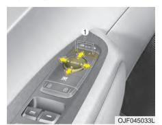
The electric remote control mirror switch allows you to adjust the position of the left and right outside rearview mirrors. To adjust the position of either mirror, press the R or L button (1) to select the right side mirror or the left side mirror, then press a corresponding point (A) on the mirror adjustment control to position the selected mirror up, down, left or right. After adjustment, press the R or L button again to prevent the inadvertent adjustment.
