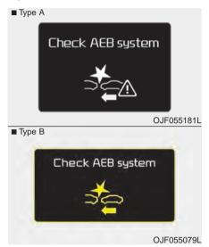
• When the AEB is not working properly, the AEB warning light ( ) will illuminate and the warning message will appear for a few seconds. After the message disappears, the master warning light (1) will illuminate. In this case, we recommend you to have the vehicle inspected by an authorized Kia dealer
