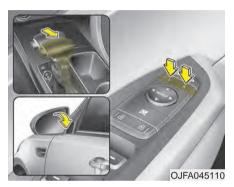
While the vehicle is moving in reverse, the outside rearview mirror(s) will move downward to aid reverse parking. According to the position of the outside rearview mirror switch (1), the outside rearview mirror(s) will operate as follows:
