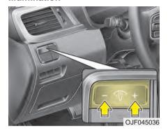
The brightness of the instrument panel illumination is changed by pressing the illumination control button ("+" or "-") when the ignition switch or Engine Start/Stop button is ON, or the taillights are turned on.
