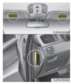
Air bag warning labels, some required by the U.S. National Highway Traffic Safety Administration (NHTSA), are attached to the sunvisor to alert the driver and passengers of potential risks of the air bag system.
