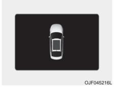
The warning message illuminates if you turn off the engine and then open the driver's door when the sunroof is open.
