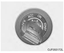
The ignition key can be removed only in the LOCK position.
