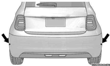
Radar Sensors Location
