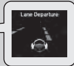
■ Tactile and visual alerts Rapid vibrations on the steering wheel and a warning display alert you that the vehicle is drifting out of a detected lane.
