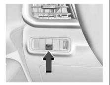
When Automatic Vehicle Hold (AVH) is turned on and the vehicle is braked to a stop, AVH prevents the vehicle from moving during the transition from brake pedal release to accelerator pedal apply. The brakes release when the accelerator pedal is applied. The brakes may also release under other conditions. Do not rely on AVH to hold the vehicle.
