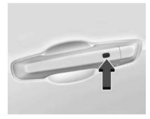
The remote key must be within 1 m (3 ft) of the liftgate or door being opened. Press the button on the front door handle to open. See *Remote Key Operation* ❖ 7.
