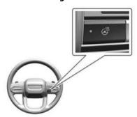
: If equipped, press to turn the heated steering wheel on or off. A light next to the button displays when the feature is turned on. The steering wheel takes about three minutes
