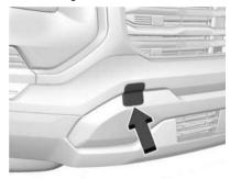
Carefully open the cover by using the small notch that conceals the front tow eye socket.
