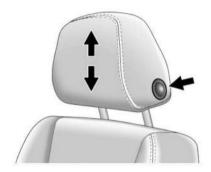
The height of the head restraint can be adjusted.
