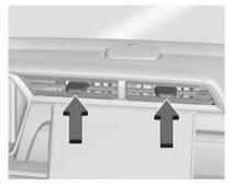
Use the air outlets in the center and on the side of the instrument panel to direct the airflow. move the center knobs on the air outlets to open or close off the airflow.
