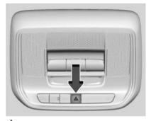
: Press this button on the overhead console to make the front and rear turn signal lights flash on and off. This warns others that you are having trouble. Press again to turn the flashers off
