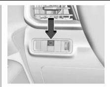
Press the switch to activate the system. The indicator flashes briefly while the system engages and stays lit when the All-Wheel Drive system is active. See All-Wheel-Drive Light ⇒ 95.
