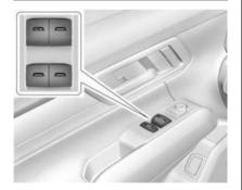
The power windows work when the vehicle is on, in accessory mode, or when Retained Accessory Power is active. See Retained Accessory Power (RAP) ⇒ 167.
