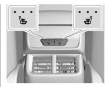
If equipped, the rear heated seat buttons are on the rear of the center console. To operate, the engine must be running.
