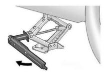
10. Raise the vehicle by turning the jack handle clockwise. Raise the vehicle far enough off the ground so there is enough room for the road tire to clear the ground.
