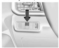
All-Wheel Drive Mode: All-Wheel Drive mode provides drive torque to all four wheels. Select All-Wheel Drive mode to improve traction and control on slippery road surfaces, such as gravel, sand, wet pavement, snow, and ice.
