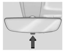
Pull the tab to turn on the display. Push the tab to turn it off. When off the mirror has automatic dimming. Adjust the mirror for a clear view of the area behind the vehicle while the display is off.
