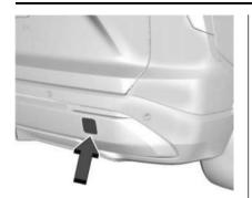
If equipped, carefully open the cover by using the small notch that conceals the rear tow eye socket.
