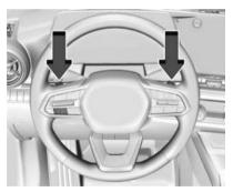
Electronic Range Select (Manual mode), allows you to select from a range of gear positions. Use this mode when driving downhill or towing a trailer to limit the top gear and vehicle speed. The shift position indicator on the Driver Information Center will display a number next to the L indicating the highest available gear.
