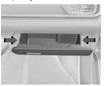
Squeeze both sides of the glove box bin inward to lower beyond the stops.
