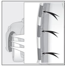
3 Insert a flathead screwdriver between the front bumper and the fender liner and then detach the claw.
