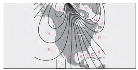
The direction display deviates from the true direction determined by the earth's magnetic field. The amount of deviation varies depending on the geographic position of the vehicle.
