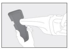
6 Reinstall the filter to the cover.
