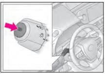
Temporarily switching to the low beams
