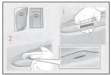
Grip the driver's door handle to unlock the door. Holding the driver's door handle for approximately 2 seconds unlocks all the doors. Grip the passenger's door
