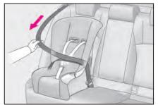
5 While pushing the child restraint system into the rear seat, allow the shoulder belt to retract until the child restraint system is securely in place.
