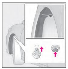
Engage the clips to the front 8 bumper to install the fender liner, and then remove the protective tape.
