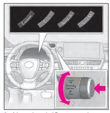
1 Normal mode/Custom mode Normal mode and custom mode are selected by pressing the Driving Mode Select switch. Each time the switch is pressed, the driving mode changes between normal mode and custom mode. When custom mode is selected, the Custom mode indicator comes on.
