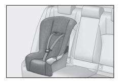
3 Run the seat belt through the child restraint system and insert the plate into the buckle. Make sure that the belt is not twisted.
