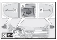
A Meter control switches Turn the Blind Spot Monitor on/off.
