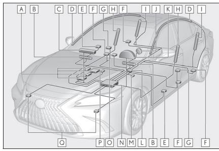
SRS airbag system components
