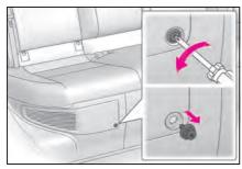
**3** Remove the air intake vent cover.
