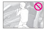
Do not attach anything to or lean anything against areas such as the dashboard, steering wheel pad and lower portion of the instrument panel. These items can become projectiles when the SRS driver, front passenger and knee airbags deploy.
