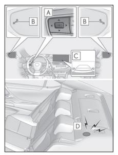
A Meter control switches Turn the RCTA function on/off. When the RCTA function is disabled, the RCTA OFF indicator illuminates.
