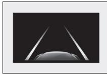
Indicates that the system is recognizing white (yellow) lines or a course<sup>\*</sup>. When the vehicle departs from its lane, the white line displayed on the side the vehicle departs from flashes orange.
