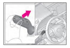
Temporarily switching to the low beams
