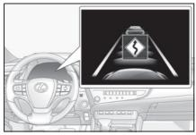
Displayed when the vehicle speed is being reduced.
