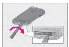
**3** Remove the depleted battery.
