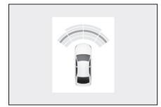
When an object is detected, a graphic will be displayed on the panoramic view monitor (if equipped).
