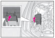
Engine compartment: type B fuse box
