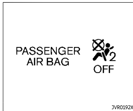
Front passenger air bag status light
