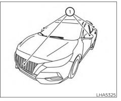
To display the multiple views, the Intelligent Around View® Monitor system uses cameras located in the front grille, on the vehicle's outside mirrors and one just above the vehicle's license plate  $\bigcirc$ .
