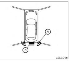
When the corner of the vehicle moves closer to an object, the corner sonar indicator A appears. When the center of the vehicle moves close to an object, the center sonar indicator B appears.
