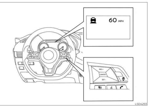
VEHICLE-TO-VEHICLE DISTANCE CONTROL MODE OPERATION The vehicle-to-vehicle distance control mode is designed to maintain a selected distance from the vehicle in front of you and can reduce the speed to match a slower vehicle ahead. The system will decelerate the vehicle as necessary and if the vehicle ahead comes to a stop, the vehicle decelerates to a standstill. However, the ICC system can only apply up to 40% of the vehicle's total braking power.
