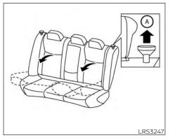
FOLDING REAR SEAT Pull the knob (a) to fold each seatback down.
