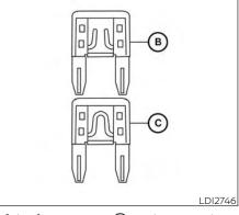
5. If the fuse is open (B), replace it with an equivalent good fuse (C).
