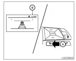
Operating vehicle-to-vehicle distance control mode
