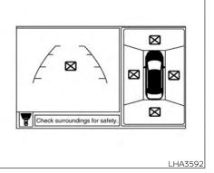
When the "[X]" icon is displayed on the screen, the camera image may be receiving temporary electronic disturbances from surrounding devices. This will not hinder normal driving operation but the system should be inspected if it occurs frequently. It is recommended that you visit a NISSAN dealer for this service.
