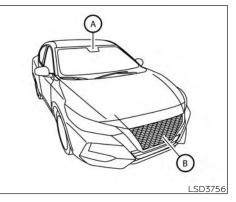
The AEB with Pedestrian Detection system uses a radar sensor located on the front of the vehicle (a) to measure the distance to the vehicle ahead in the same lane. For pedestrians, the AEB with Pedestrian Detection system uses a camera installed behind the windshield (A) in addition to the radar sensor.
