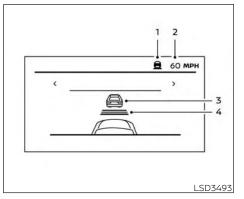
Vehicle-to-vehicle distance control mode display and indicators
