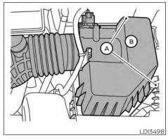
The viscous paper type filter element should not be cleaned and reused. Replace it according to the maintenance log shown in the "Maintenance and schedules" section of this manual.
