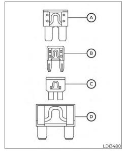
Four types of fuses are used. Type ( $\triangle$ ) is used exclusively in the passenger compartment fuse box.
