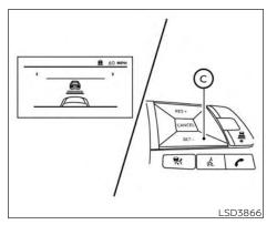
To set cruising speed, accelerate your vehicle to the desired speed, push the SETswitch ③ and release it. The ICC system set indicator (green), vehicle ahead detection indicator, set distance indicator and set vehicle speed indicator ④ will come on. Take your foot off the accelerator pedal. Your vehicle will maintain the set speed. When the SET- switch is pushed under the following conditions, the system cannot be set and the ICC indicators will blink for approximately 2 seconds:
