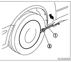
Removing wheel cover (if so equipped)
