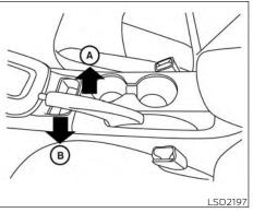
HAND TYPE (if so equipped) **To engage:** Pull the lever up (A).
