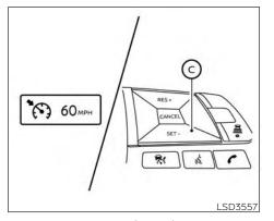
To set cruising speed, accelerate your vehicle to the desired speed, push the SET- ③ switch and release it. (The color of the cruise indicator changes to green and set vehicle speed indicator comes on.) Take your foot off the accelerator pedal. Your vehicle will maintain the set speed.
