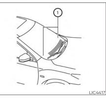
Be sure you do not put anything on top of the autolight sensor located in the top side ① of the instrument panel. The autolight sensor controls the autolight; if it is covered, the autolight sensor reacts as if it is dark out and the headlights will illuminate. If this occurs while parked with the engine off and the ignition switch placed in the ON position, your vehicle's battery could become discharged.
