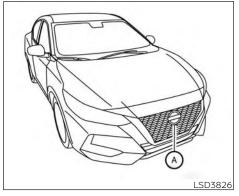
The I-FCW system uses a radar sensor A located on the front of the vehicle to measure the distance to the vehicle ahead in the same lane.
