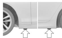
The jacking points are located at the indicated positions.
