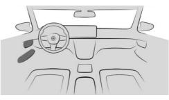
The central locking buttons are located on the front door.
