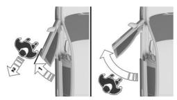
If the person opening the door is detected as an obstacle, the door stops, arrow 1. If
