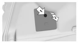
Turn the screw cap in the cover by 90°, arrow 1, and fold down the trim panel, arrow 2.
