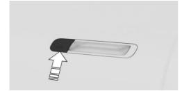
Hold the near field communication antenna of the smartphone directly and centered on the external door handle of the driver's door. The position of the near field communication antenna depends on the smartphone model.
