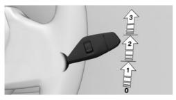
Press the lever up until the desired position is reached.
