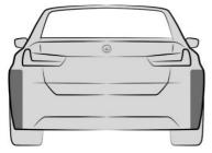
The radar sensors are located on the side in the rear bumper.
