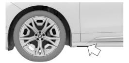
The light source is located in the position indicated. Keep the light source clean and unobstructed.
