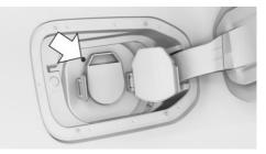
The charging status is indicated on the indicator light on the charging socket.
