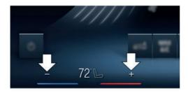
You can set the desired temperature for driver and front passenger individually on the menu bar.
