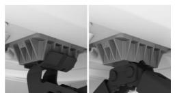
3. Extend the jack by turning the jack crank handle or lever clockwise.
