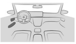
The seat adjustment menu button is located on the front door.
