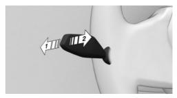
To reactivate the Automatic High Beam Assistant, press the turn signal lever up, arrow 1.
