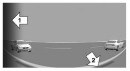
Depending on the direction of travel, the view to the front or back is displayed in the camera image. The respective boundary area, arrow 1, in the camera image flashes red if vehicles are detected by the sensors.
