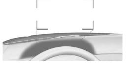
Head-up display views are projected onto the windshield using protective glass. The protective glass is located between the steering wheel and windshield.
