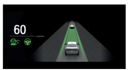
An example of active Driver Assistance: Indicator and warning lights for Distance Control and Assisted Driving Mode are displayed. At the same time, the Distance Control is animated in Assisted View.
