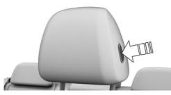
Press the button and push the head restraint forward or backward.
