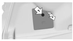
The onboard vehicle tool kit is located in the left storage compartment of the cargo area. Turn the cover lock, arrow 1, and fold out the trim panel, arrow 2.
