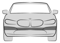
The ultrasonic sensors of the parking assistance systems are located in the front bumper.
