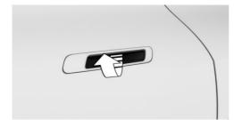
Press and hold the button in the recessed grip to unlock the vehicle and open the rear door.
