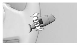
Turn the thumbwheel on the wiper lever.
