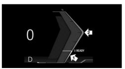
Needle in the area of arrow 1: display of the energy recovered by coasting or when decelerating.
