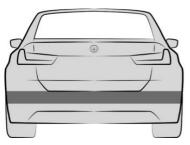
The ultrasonic sensors of the parking assistance systems are located in the rear bumper.
