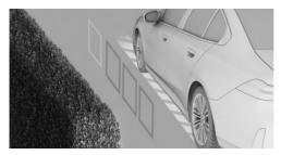
To protect the sides of the vehicle, obstacle markings are displayed on the sides of the vehicle.
