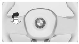
The shift paddle for the Sport Boost function is located on the steering wheel.
