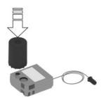
2. Turn the sealant bottle clockwise by 90° to the stop.
