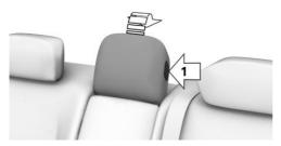
Press button, arrow 1, and fold the head restraint back.
