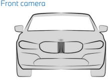
The front camera is located in the radiator grille.
