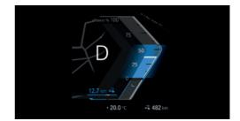
The efficient range of the power gauge is colored blue. Additionally, the bonus range will be displayed.
