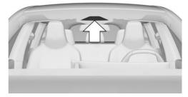
The camera behind the windshield is located near the interior mirror.
