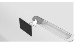
Hold activated Key Card directly on the center of the external door handle of the driver's door.
