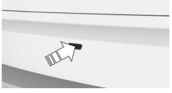
▷ Unlock the vehicle and then press the button on the trunk.
