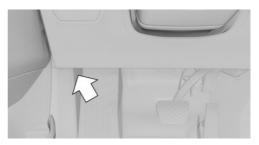
There is an onboard diagnostic port for reading out vehicle data on the left side of the vehicle.
