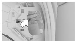
5. Pull the object out of the opening again. The glove compartment opens.
