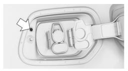
The charging cable release key is located next to the charging socket.
