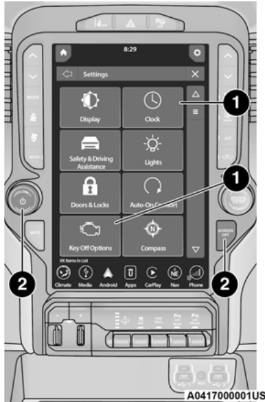
Uconnect 4C NAV With 12-inch Display Buttons On The Touchscreen And Buttons On The Faceplate
