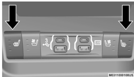
Rear Heated Seat Switches
