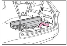
5 Loosen the center fastener that secures the compact spare tire.
