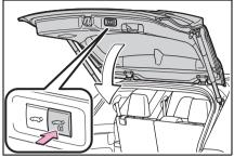
2 While the buzzer is sounding, move away from the back door.
