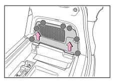
3 Disengage the 5 claws and pull the cover to remove it.
