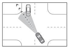
When turning left/right and a pedestrian or bicycle is detected
