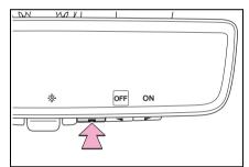
2 Press represented on the original of the enable ("ON")/disable ("OFF") the automatic anti-glare function.
