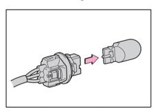
3 Install a new light bulb and then install the bulb base to the light unit by inserting it and turning it clockwise.
