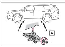
4 Install the wheel nut wrench to the jack handle.
