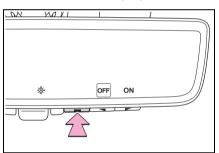
2 Press ro ro to enable ("ON")/disable ("OFF") the automatic anti-glare function.
