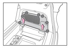
**3** Disengage the 5 claws and pull the cover to remove it.
