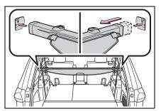
4 Pull out the luggage cover and hook it onto the anchors.
