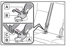
**3** Stow the plate C and A in the holder on the roof.
