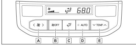
A Adjust the rear seats fan speed setting
