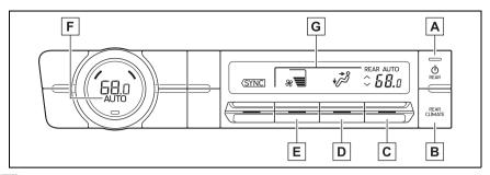
A Rear air conditioning system on/off switch
