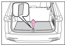
2 To fix the center deck board. at the upright position, using the straps of the back side of the third-row seats, fasten the velcro tapes to the underside of the center deck board
