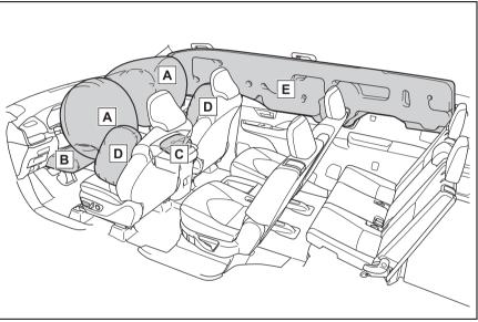
A SRS driver airbag/front passenger airbag
