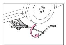
4 Securely tighten the wheel nuts two or three times in the order shown in the illustration using a wheel nut wrench. Vehicles with wheel locks: Tighten the wheel lock using the wheel lock key after tightening the other wheel nuts.
