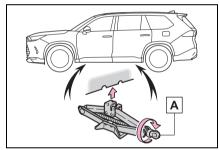
Install the wheel nut wrench to the jack handle.
