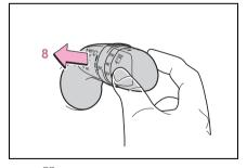
Pulling the lever operates the wipers and washer.
