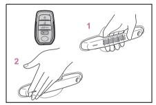
Grip the driver's door handle to unlock the door. Holding the driver's door handle for approximately 2 seconds unlocks all the doors. Grip any passenger door handle to unlock all the doors.\*
