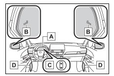
A Multi-information display Turning the safe exit assist on/off. If collision with a door is likely and the door is opened, the door will be displayed on the multi-information display. Also, if a door is opened when an outside rear view mirror indicator is illuminated, a buzzer will sound as a warning.
