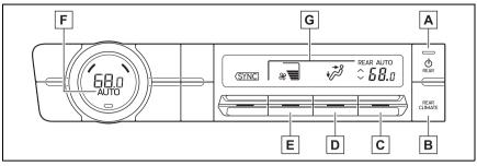
A Rear air conditioning system on/off switch
