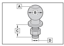
A Trailer ball load rating Matches or exceeds the gross
