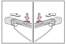
**3** To install the luggage cover unit, with the lock release buttons facing upward, insert one end into the recess, then Interior features
