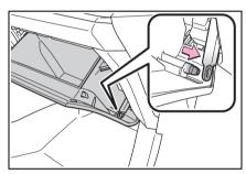
3 Push in each side of the glove box to disconnect the claws. Then pull out the glove box and disconnect the lower claws.
