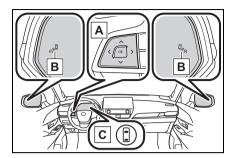
A Meter control switches Turning the Blind Spot Monitor on/off.
