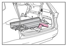
5 Loosen the center fastener that secures the compact spare tire.
