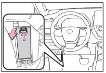
3 Remove the fuse with the pullout tool.Only some fuses can be removed using the pullout tool.
