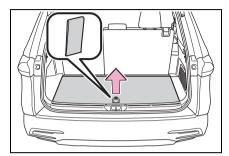
2 To fix the center deck board at the upright position, using the straps of the back side of the third-row seats, fasten the velcro tapes to the underside of the center deck board.
