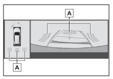
A Pedestrian detection icon Displayed automatically when a pedestrian is detected behind the vehicle.
