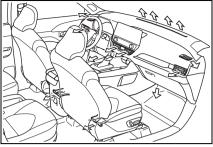
Adjusting the air flow direction and opening/closing the air outlets
