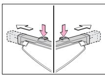
3 To install the luggage cover unit, with the lock release buttons facing upward, insert one end into the recess, then
