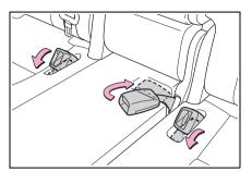
3 Pass the outer seat belts through the seat belt hangers and secure the seat belt plates.
