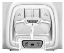
The dome lights and dome light controls are in the overhead console.
