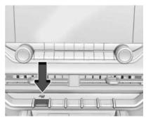
Turn the Tow/Haul Mode on and off by pressing the button on the center stack. When the Tow/Haul Mode is enabled, a light on the instrument cluster will come on
