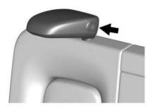
The rear seat outboard head restraints are designed to be folded.
