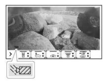
Touch the symbol on the lower-left of the infotainment display to activate the washer.
