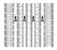
Treadwear indicators are one way to tell when it is time for new tires. Treadwear indicators appear when the tires have only 1.6 mm (1/16 in) or less of tread remaining. See *Tire Inspection* ⇔ 279 and *Tire Rotation* ❖ 279.
