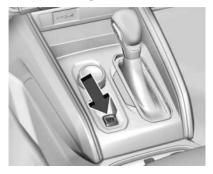
The Electric Parking Brake can always be applied, even if the vehicle is off. In case of insufficient electrical power, the Electric Parking Brake cannot be applied or released. To prevent draining the battery, avoid unnecessary repeated cycles of the Electric Parking Brake.
