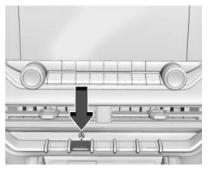
The Auto Stop/Start feature can be disabled and enabled by pressing (A). Stop/Start is enabled each time you start the vehicle.
