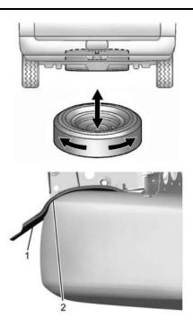
7. Make sure the tire is stored securely and flush in the radius (2) of the spare tire support bracket (1). Push, pull, and then try to turn the tire. If the tire moves, use the wheel wrench to tighten the cable. Repeat this tightness check procedure when checking the spare tire pressure according to the scheduled maintenance information or any time the spare tire is handled due to service of other components.
