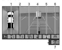
Touch the camera view buttons along the bottom of the infotainment display to access each view (if equipped):
