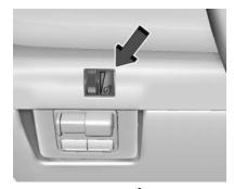
Rotate this thumbwheel  $\mathcal{E}^{\mathfrak{F}}$  up or down to adjust the brightness of all illuminated controls. The thumbwheel is on the instrument panel to the left of the steering wheel.
