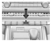
Press the button to make the front and rear turn signal lights flash on and off. This warns others that you are having trouble. Press again to turn the flashers off
