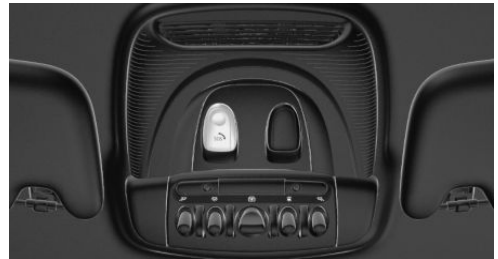
SOS button in the roofliner
