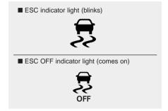
When the Engine Start/Stop button is pressed to the ON position, the ESC indicator light illuminates, then goes off if the ESC system is operating normally.
