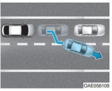
When driving in stop-and-go traffic, and a stopped vehicle in front of you merges out of the lane, the system may not immediately detect the new vehicle that is now in front of you. In this case, you must maintain a safe braking distance, and if necessary, depress the brake pedal to reduce your driving speed in order to maintain a safe distance.
