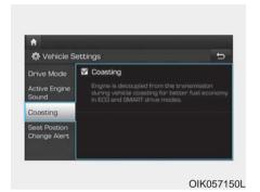
Select 'Settings → Vehicle settings → Coasting' on the audio or AVN screen. Turn the function ON and the ECO Coasting function will activate.
