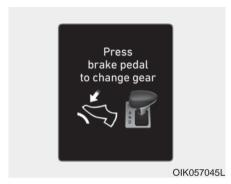
The message appears on the LCD display when the brake pedal is not depressed while shifting the gear.
