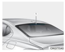
If the high mounted stop lamp (LED) (1) does not operate, have the system be checked by an authorized retailer of Genesis Branded products.
