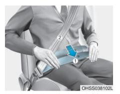
You should place the lap belt (1) portion across your hips and the shoulder belt (2) portion across your chest. The seat belt automatically adjusts to the proper length after the lap belt portion is adjusted manually so that it fits snugly around your hips. If you lean forward in a slow, easy motion, the seat belt will extend and move with you.
