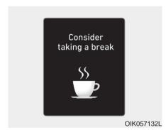
The "Consider taking a break" message appears on the LCD display and a warning sounds in order to suggest the driver to take a break, when the driver's attention
