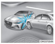
Front air bags may not inflate in side impact collisions, because occupants move in the direction of the collision, and thus in side impacts, front air bag deployment would not provide additional occupant protection.
