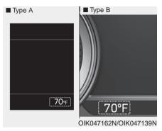
This gauge indicates the current outside air temperature by 1°F (1°C).
