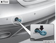
If towing is necessary, we recommend you have it done by an authorized retailer of Genesis Branded products or a commercial tow truck service. If a towing service is not available in an emergency, your vehicle may be temporarily towed using a cable or chain secured to the emergency towing hook at the front (or rear) of the vehicle.
