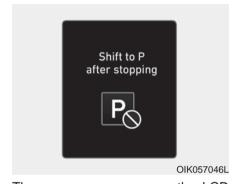
The message appears on the LCD display when the gear is shifted to P (Park) while the vehicle is moving. Stop the vehicle before shifting to P (Park).
