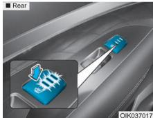
While the engine is running, push either of the switches to warm the driver's seat or front passenger's seat (and/or rear passenger's seat).
