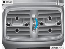
The outlet vents can be opened ( $\circledast$ ) or closed ( $\bigcirc$ ) separately using the thumbwheel.
