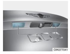
If the license plate lamp (LED) (1) does not operate, have the system be checked by an authorized retailer of Genesis Branded products.
