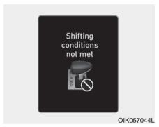
The message appears on the LCD display when engine rpm is too high, or when driving speed is too fast to shift the gear.
