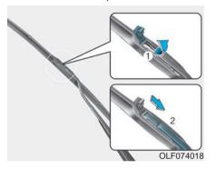
2. Lift up the wiper blade clip (1). Then pull down the blade assembly (2) and remove it.
