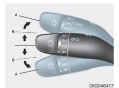
To signal a turn, push down on the lever for a left turn or up for a right turn in position (A). To signal a lane change, move the turn signal lever slightly and hold it in position (B). The lever will return to the OFF position when released or when the turn is completed.
