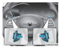
The paddle shifter is available when the shift lever is in the D (Drive) position.
