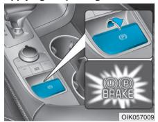
To apply the EPB (Electronic Parking Brake):
