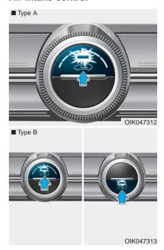
This button is used to select the outside (fresh) air position or recirculated air position.
