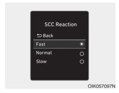
The sensitivity of vehicle speed when following the front vehicle to maintain the set distance can be adjusted. Go to the 'User Settings  $\rightarrow$  Driver Assistance  $\rightarrow$  SCC Reaction  $\rightarrow$  Fast/Normal/Slow' on the LCD display. You may select one of the three stages you prefer.
