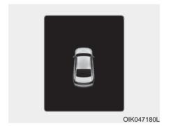
This warning is displayed if you turn off the engine when any window is open.
