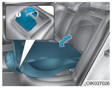
4. Pull up the seatback folding lever (1), then fold the seat toward the front of the vehicle.
