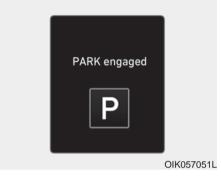
The message appears on the LCD display when the P (Park) position is engaged.
