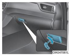
When leaving keys with parking lot and valet attendants, the following procedures will ensure your vehicle's glove box compartment can only be opened with the mechanical key.
