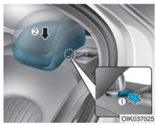
Lower the rear head restraints to the lowest position by pushing and holding the release button (1) and pushing down on the headrest (2).
