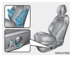
Seat back bolster adjustment (for driver's seat, if equipped)
