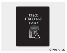
The message appears on the LCD display when there is problem with the P RELEASE button.
