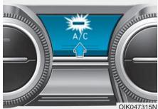
Push the A/C button to manually turn the system on (indicator light will illuminate) and off.
