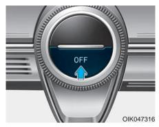
Push the OFF button to turn the climate control system off. You can still operate the mode and air intake buttons as long as the Engine Start/Stop button is in the ON position.
