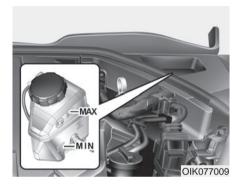
Check the fluid level in the reservoir periodically. The fluid level should be between MAX and MIN marks on the side of the reservoir.
