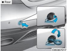
Remove the hole cover pressing the lower part of the cover on the front or rear bumper.
