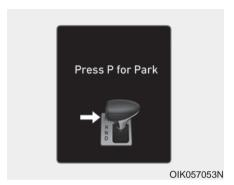
The message appears on the LCD display to inform the driver to press the P button to shift to P (Park) when the driver moves the shift lever upward even though the gear is in R (Reverse).
