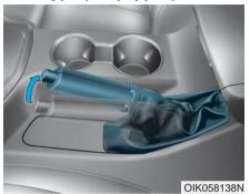
Check the stroke of the parking brake by counting the number of "clicks" heard while fully applying it from the released position. Also, the parking brake alone should securely hold the vehicle on a fairly steep grade. If the stroke is more or less than specified, have the parking brake adjusted by an authorized retailer of Genesis Branded products.
