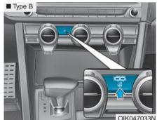
When the Engine Start/Stop button is in the ON position, press the heated steering wheel switch to warm the steering wheel.  Each time you push the switch, the temperature setting changes as follows:
