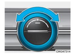
The fan speed can be set as desired by turning the fan speed control knob. Turn the knob to the right for higher fan speed.
