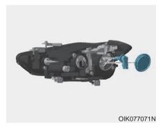
Disconnect the bulb socket-connector.
