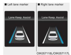
A visual warning appears on the cluster LCD display. Either the left lane marker or the right lane marker in the cluster LCD display will blink depending on which direction the vehicle is veering. Also, the steering wheel will vibrate (if equipped).
