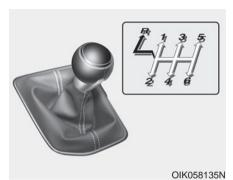
The manual transmission has 6 forward gears. The transmission is fully synchronized in all forward gears so shifting to either a higher or a lower gear is easily accomplished.
