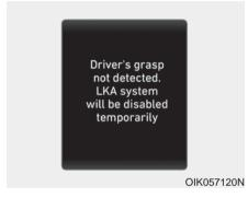
If the driver still does not have their hands on the steering wheel after the message "Keep hands on steering wheel", the system will not control the steering wheel and warn the driver only when the driver crosses the lane markers.
