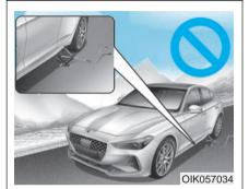
Never start or run the engine while an AWD vehicle is raised on a jack. The vehicle can slip or roll off of a jack causing serious injury or death to you or those nearby.
