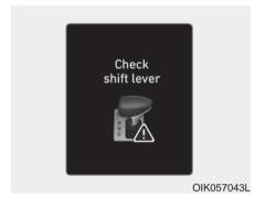
The message appears on the LCD display when there is a malfunction with one of the key transmission shifter components.
