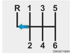
This manual transmission is designed with a detent to differentiate 1st and R (Reverse) gear. To shift into reverse, you must shift past 1st gear and the detent in order to get into the R (Reverse) gear gate.
