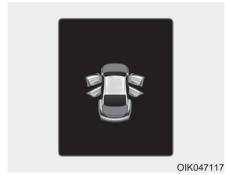
This warning is displayed if any door or the hood or the trunk is left open. The warning will indicate which door is open in the display.
