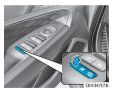
The driver can disable the power window switches on the rear passenger doors by pressing the power window lock switch. The indicator will be illuminated.
