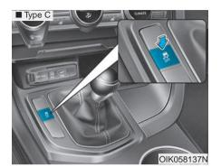
The Electronic Stability Control (ESC) system helps to stabilize the vehicle during cornering maneuvers. ESC checks where you are steering and where the vehicle is actually going. ESC applies braking pressure to any one of the vehicle's brakes and intervenes in the engine management system to assist the driver with keeping the vehicle on the intended path. It is not a substitute for safe driving practices. Always adjust your speed and driving to the road conditions.
