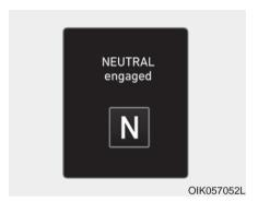
The message appears on the LCD display when the N (Neutral) position is engaged.
