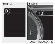
This indicator displays the gear position of the shift lever.
