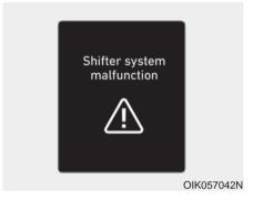
The message appears on the LCD display when the transmission or the shift lever does not properly operate in the P (Park) position.
