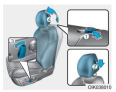
To reinstall the head restraint:
