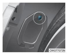
Remove the service cover (1) under the wheel housing by pushing out the retainer clip with a slim tool. If it is difficult to remove the service cover because of the tire, steer the tire inward.
