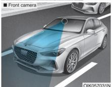
In order for the FCA system to operate properly, always make sure the sensor cover or sensor is clean and free of dirt, snow, and debris.
