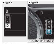
Shift indicator pop-up (if equipped) The pop-up indicates the current gear position displayed in the cluster for about 2 seconds when shifting into other positions (P/R/N/D).
