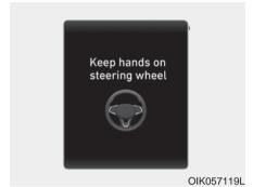
If the driver takes their hands off the steering wheel for several seconds while the LKA system is activated, the system will warn the driver.
