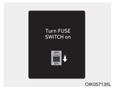
This warning message is displayed if the fuse switch located on the fuse box under the steering wheel is OFF.
