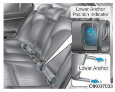
The lower anchor position indicator symbols are located on the left and right rear seat backs to identify the position of the lower anchors in your vehicle (see arrows in illustration).
