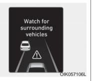
If the vehicle ahead (vehicle speed: less than 20 mph (30 km/h)) disappears to the next lane, the warning chime will sound and a message "Watch for surrounding vehicles" will appear. Adjust your vehicle speed for vehicles or objects that can suddenly appear in front of you by depressing the brake pedal.
