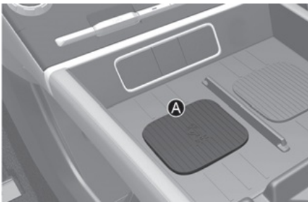
[A] Vehicle authentication pad (Wireless charging pad)
