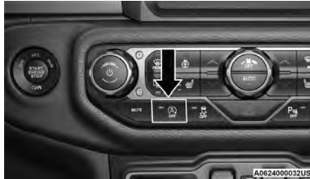
Stop/Start OFF Switch
