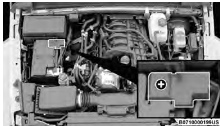
Positive (+) Battery Post – Gas Engine
