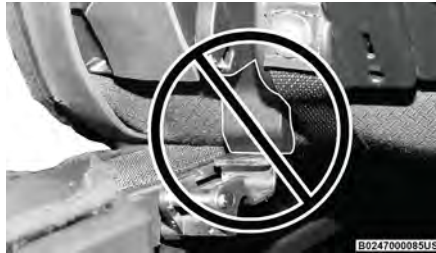
Incorrectly Seated Retainer
