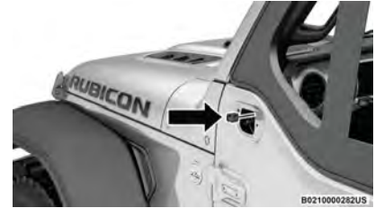
Wiring Harness Location
