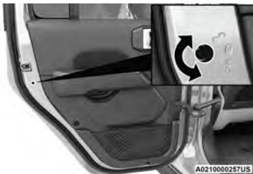
Child-Protection Door Lock Location
