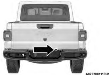
Access Hole Location
