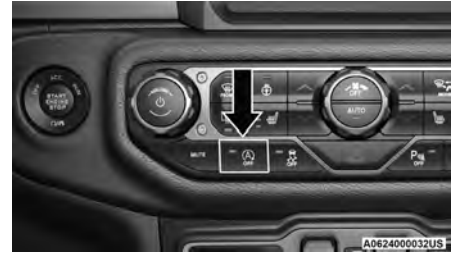
Stop/Start OFF Switch
