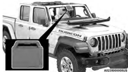
Protective Cover Installed
