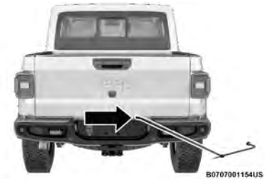
Inserting The Extensions Into The Winch Mechanism Access Hole
