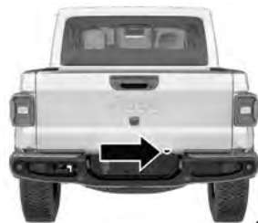
Winch Mechanism Access Hole
