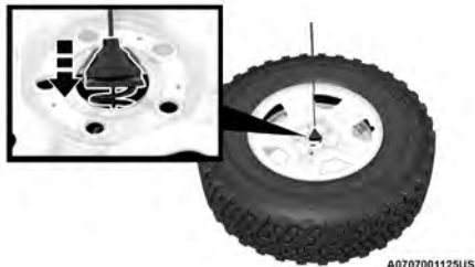
Reinstalling The Retainer
