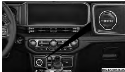
Front Power Outlet
