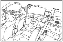
Adjusting the air flow direction and opening/closing the air outlets
