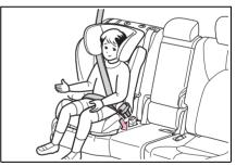
Removing a child restraint system installed with a seat belt
