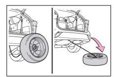
5 Before raising the tire, make sure that the hoist assembly is perpendicular to the wheel opening. (Try to place the tire directly beneath the vehicle, near where the wire cable is hanging from.)
