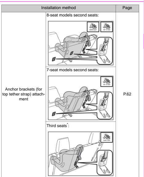
\*: The third seats are not equipped with Child restraint LATCH anchors.
