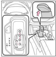
While the engine switch is in ON and the brake pedal depressed<sup>\*</sup>, shift the shift lever while pushing the shift release button on the shift knob.
