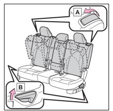
Pull the seatback folding lever to unlock the seatback. The seatback will be folded down.
