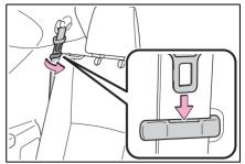
3 Lower the center head restraint to the lowest position. (→P.140)
