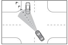
When you turn right/left, pedestrian is detected in the forward direction and estimated to enter your vehicle's path (bicyclists are not detected.)
