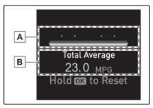
A Current fuel consumption Displays instantaneous current fuel consumption.
