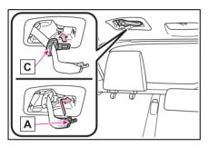
Adjusting the seat belt shoulder anchor height (front seats)
