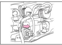
4 Turn the bulb base counterclockwise and remove it.
