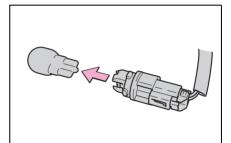
4 Install a new light bulb, and then install the bulb base to the light unit by inserting it and turning it clockwise.
