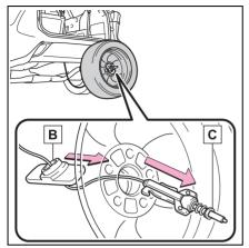
Fully depress the secondary latch A and install the bracket B to the hoist assembly C.
