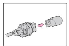
3 Install a new light bulb, and then install the bulb base to the light unit by inserting it and turning the bulb base clockwise.
