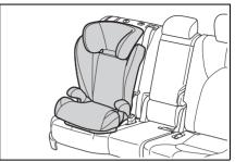
4 Sit the child in the child restraint system. Fit the seat belt to the child restraint system according to the manufacturer's instructions and insert the plate into the buckle. Make sure that the belt is not twisted.
