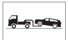
Release the parking brake. Turn automatic mode off. (→P.205) ► From the front (AWD models)
