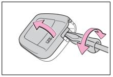
3 Remove the depleted battery.
