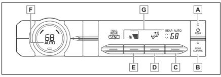
A Rear air conditioning system on/off switch
