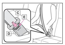
2 To release plate A, insert the mechanical key (→P.110) or plate C into the hole on buckle B.
