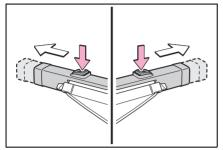
3 To install the luggage cover unit, with the lock release buttons facing upward, insert one end into the recess, then compress the other end and insert it into the other recess.
