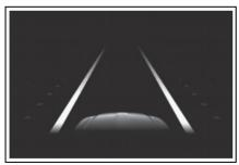
Indicates that the system is recognizing white (yellow) lines or a course<sup>\*</sup>. When the vehicle departs from its lane, the white line displayed on the side the
