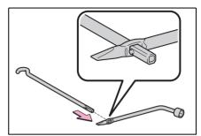
6 Connect the jack handle to the adapter socket. Turn the jack handle counterclock-wise.
