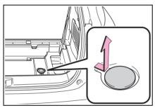
4 Attach the adapter socket to the spare tire clamp bolt.
