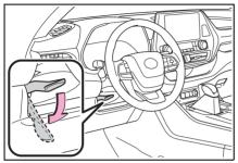
2 Adjust to the ideal position by moving the steering wheel horizontally and vertically.
