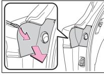
2 Remove the securing 2 screws and light unit.
