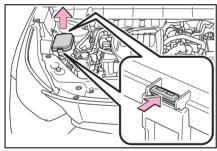
Engine compartment: type B fuse box
