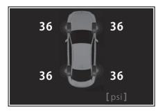
If the tire pressure drops below a predetermined level, the driver is warned by a screen display and a warning light. (→P.433)
