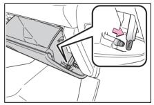
3 Push in the glove box on the vehicle's outer side to disconnect the claws. Then pull out the glove box and disconnect the lower claws.
