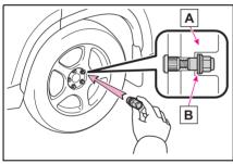
When replacing an aluminum wheel with a steel wheel, tighten the wheel nuts until the tapered portion  $\boxed{A}$  comes into loose contact with the disc wheel seat  $\boxed{B}$ .
