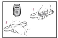
Grip the driver's door handle to unlock the door. Holding the driver's door handle for approximately 2 seconds unlocks all the doors. Grip the front passenger's door handle to unlock all the doors.\*
