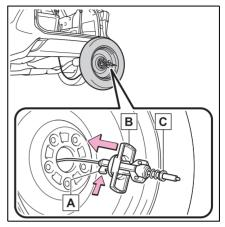
9 Tilt the bracket B and pass it through the wheel opening.
