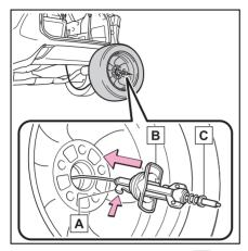
9 Tilt the holding bracket B so that it can easily be passed through the wheel opening. After passing the holding bracket through the wheel opening, remove the hoist assembly C.
