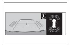
• Example (Panoramic view monitor) (if equipped): Vehicles are approaching from both sides of the vehicle
