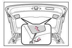
2 Turn the bulb base counterclockwise and remove it.
