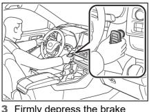
3 Firmly depress the brake pedal and check that a is shown on the multi-information display.
