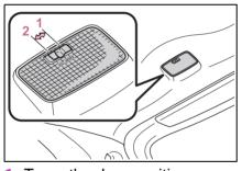
**1** Turns the door position on The rear interior light turns on/off together the front interior lights. When a door is opened while the front and rear interior light door position is on, the lights turn on.
