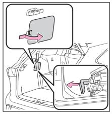
Using the lever to open the fuel filler door may not allow for an adequate reduction in fuel tank pressure before refueling. To prevent fuel from spilling out, turn the cap slowly when removing it. During refueling, fuel may spill out from the filler opening due to air being discharged from inside the fuel tank. Therefore, fill the fuel tank carefully and slowly.
