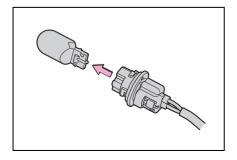
6 Install a new light bulb, and then install the bulb base to the light unit by inserting it and turning it clockwise.
