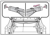
4 Pull out the luggage cover and hook it onto the anchors.
