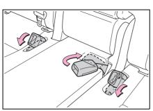
3 Pass the outer seat belts through the seat belt hangers and secure the seat belt plates.
