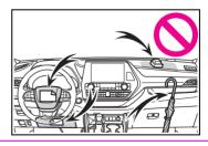
Do not attach anything to areas such as a door, windshield, side windows, front or rear pillar, roof side rail and assist grip.
