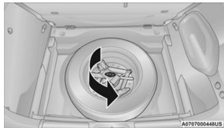
Removing Jack And Spare Tire Fastener
