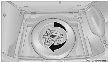
Reinstalling Jack and Tire Fastener
