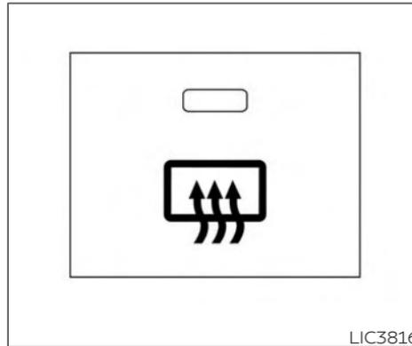
To defrost the rear window glass and outside mirrors, place the ignition switch in the ON position and push the rear window defroster switch on. The rear window defroster indicator light comes on. Push the switch again to turn the defroster off.
