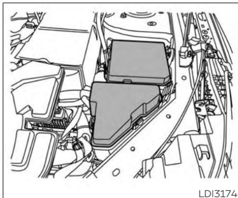
3. Remove the fuse box cover by pushing the tabs and lifting the cover up.
