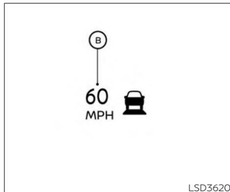
When passing another vehicle, the set speed indicator (B) flashes when the vehicle speed exceeds the set speed. The vehicle ahead detection indicator turns off when the area ahead of the vehicle is open. When the pedal is released, the vehicle returns to the previously set speed. Even though your vehicle speed is set in the ICC system, you can depress the accelerator pedal when it is necessary to accelerate your vehicle rapidly.
