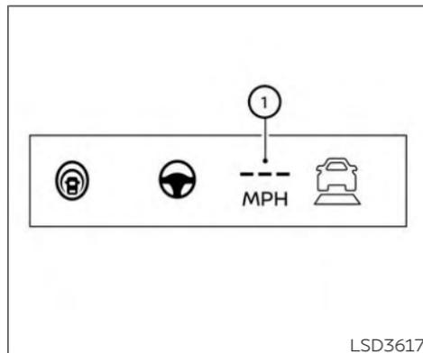
When the SET- switch is pushed under the following conditions, the ProPILOT Assist system cannot be set and the set vehicle speed indicator **1** blinks for approximately 2 seconds:
