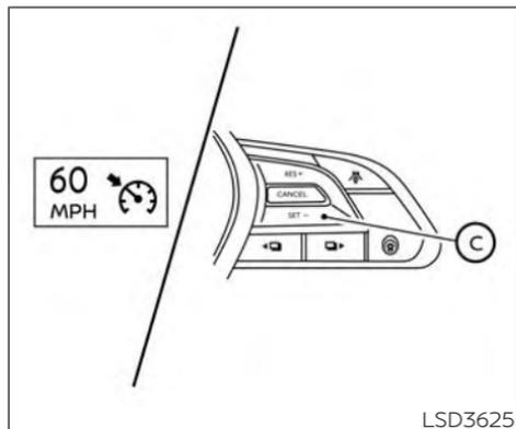
To set cruising speed, accelerate your vehicle to the desired speed, push the SET-
