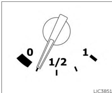
**Refill the fuel tank once the Low Fuel warning indicator in the vehicle information display illuminates as indicated by
