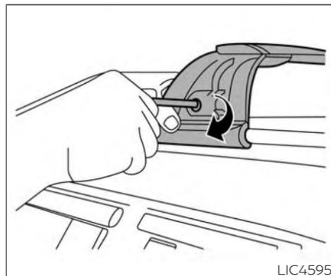
8. Tighten both the driver and passenger side clamping screw.
