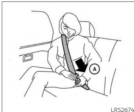
2. Slowly pull the seat belt out of the retractor and insert the tongue into the buckle
