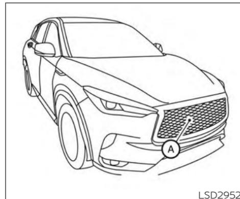
The PFCW system uses a radar sensor
