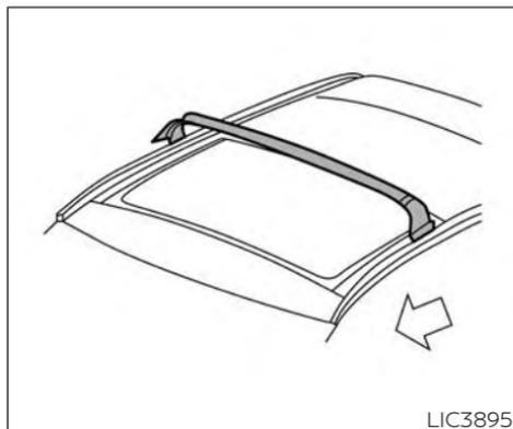
6. Align the pins on the passenger and driver side inner clamp with the holes in the roof side rails.
