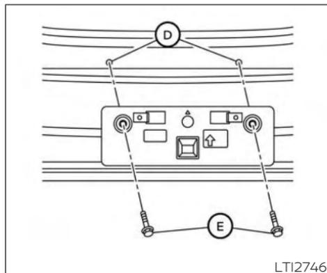
7. Insert two screw grommets (D) into the fascia.
