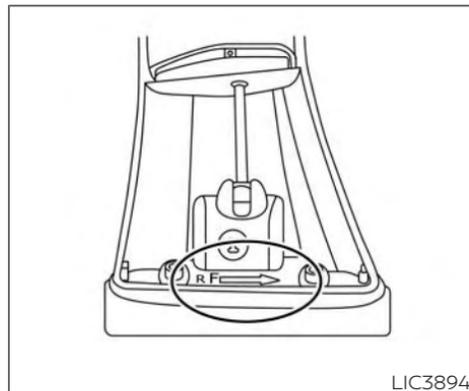
5. Determine crossbar orientation by locating the arrow that points to the front of the vehicle.
