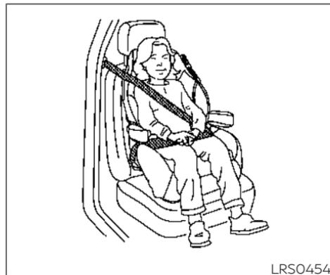
3. The booster seat should be positioned on the vehicle seat so that it is stable.
