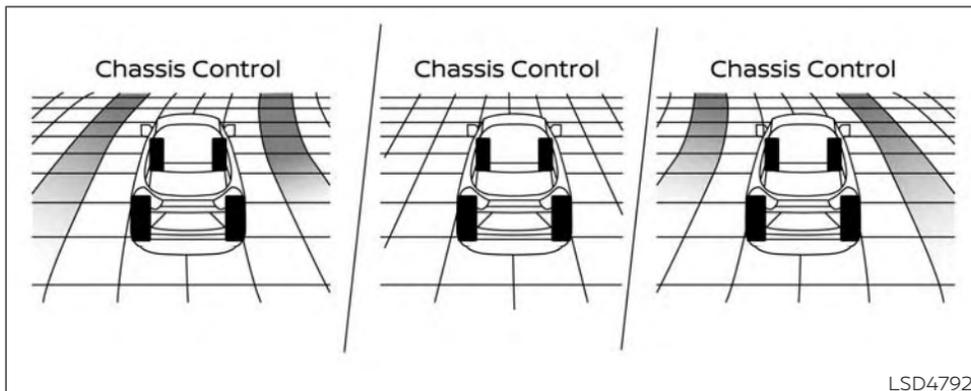
When the Active Trace Control is operated and the "Chassis Control" mode is selected in the vehicle information display, the Active Trace Control graphics are shown in the vehicle information display.
