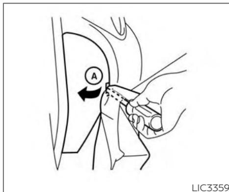
The extended storage switch is used when shipping the vehicle. It is located in the fuse panel on the driver's side of the instrument panel. If any electrical equipment does not operate, ensure the extended storage switch is pushed fully in place, as shown.
