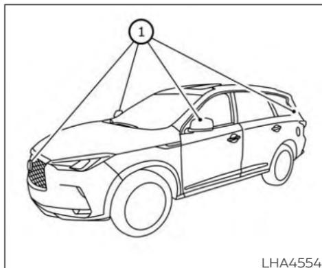
If dirt, rain or snow accumulates on any of the cameras ①, the Around View® Monitor may not display objects clearly. Clean the camera by wiping with a cloth dampened with a diluted mild cleaning agent and then wiping with a dry cloth.
