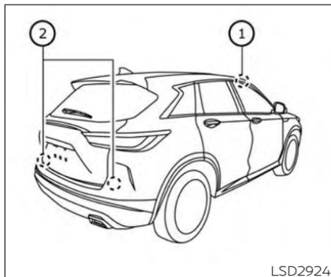
The BSI system uses radar sensors ② installed near the rear bumper to detect other vehicles in an adjacent lane. In addition to the radar sensors, the BSI system uses a camera ① installed behind the windshield to monitor the lane markers of your traveling lane.
