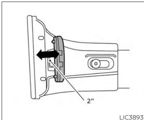
4. Open the clamp approximately two inches to minimize potential scratching of the roof side rails.
