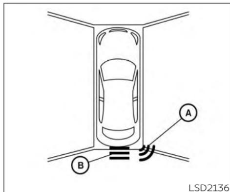
When the corner of the vehicle moves closer to an object, the corner sonar indicator (A) appears. When the center of the vehicle moves close to an object, the center sonar (if so equipped) indicator (B) appears.
