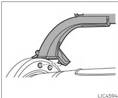
7. While holding the inner clamp, use an allen key to tighten the clamping screw.
