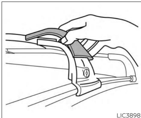
10. Assemble the plastic cover. Slide the cover over the crossbar.
