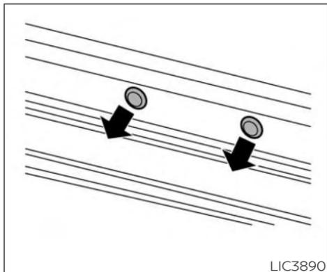
1. Manually remove the protective covers from the roof side rails.
