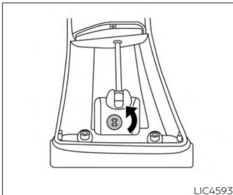
3. Use an allen key to loosen the clamp screw.
