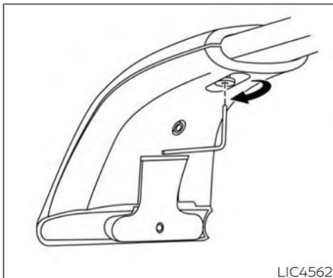
9. Tighten both the driver and passenger side shoulder screw.
