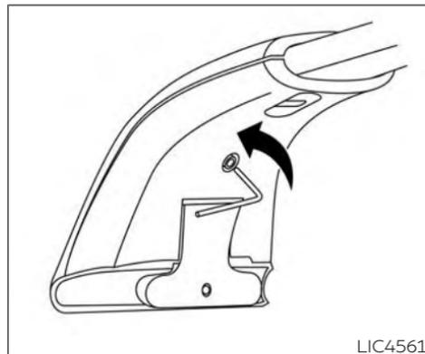
2. Using an allen key, untighten the screw to remove the plastic cover.
