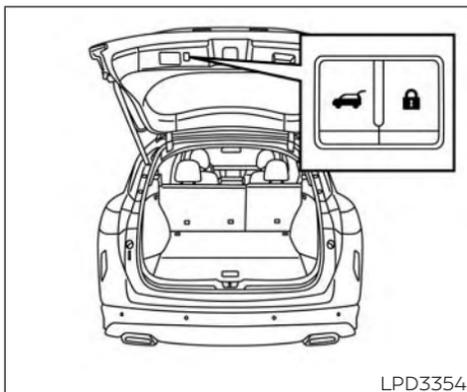
3. Push and hold the power liftgate close switch
