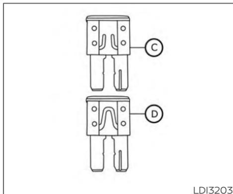
5. If the fuse is open (C), replace it with an equivalent good fuse (D).
