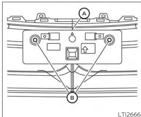
2. Cross-car alignment can be done using centerline in bracket and centerline in fascia **A**.
