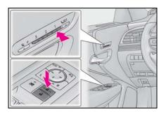
4 While pressing the recalled button, press and hold the door lock switch (either lock or unlock) until the buzzer sounds.
