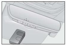
Point the remote control transmitter for the device at the rear view mirror, 1 to 3 in. (25 to 75 mm) from the HomeLink® buttons.
