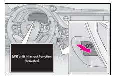
While the vehicle is stopped, press and hold the parking brake switch until a message is shown on the multi-information display.
