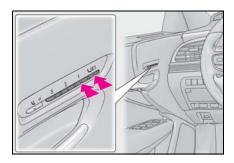
**4** While pressing the "SET" button, or within 3 seconds after the "SET" button is pressed, press button "1", "2" or "3" until the buzzer sounds.
