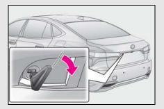
Turn the mechanical key clockwise to open.
