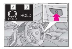
Press the brake hold switch to turn the system on
