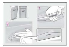
1 Grip the driver's door handle to unlock the door. Holding the driver's door handle for approximately 2 seconds unlocks all the doors. Grip any passenger door handle to unlock all the doors.\*
