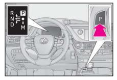
Fully stop the vehicle and set the parking brake, and then press the P position switch.
