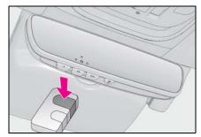
Press and hold the handheld transmitter button until the HomeLink<sup>®</sup> indicator light changes from slowly flashing orange to rapidly flashing green (rolling code) or continuously lit green (fixed code), then release the button.
