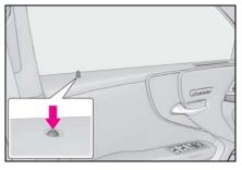
Push down the inside lock button to lock the door.
