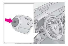
Press the Automatic High Beam switch.
