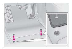
1 Insert the retaining hooks (clips) into the floor mat eyelets.
