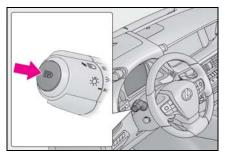
1 Press the Automatic High Beam switch.
