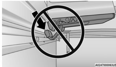
Improper Clamp Position
