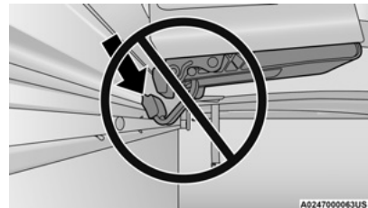
Improper Clamp Position
