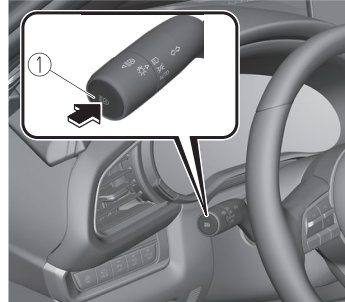
1. High beam control switch
