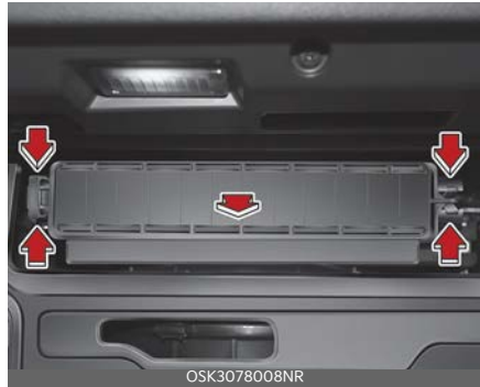
3. Replace the climate control air filter.
