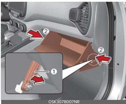
2. With the glove box open, pull the support strap (1). Push in Both sides (2) of the glove box as shown.
