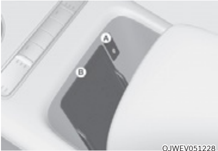
[A] : Indicator light, [B] : Charging pad
