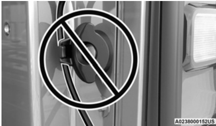
Incorrectly Seated Tailgate Strap
