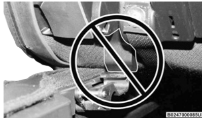
Incorrectly Seated Retainer
