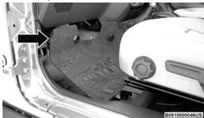
Front Carpet Pulled Away
