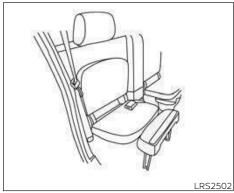
To access the jump seat extension (passenger's side only) (a) on the jump seat, pull up (b) on the extension to unfold it to the open position. Then unfold the two support legs (a) and lower the jump seat to the full open seating position.
