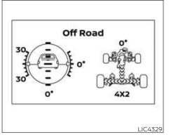
OFF-ROAD AND 4-WHEEL DRIVE (4WD) MONITOR (if so equipped)
