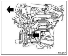
3.8L 6 cylinder (VQ38DD engine model) **ENGINE SERIAL NUMBER**
