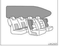
Front seat-mounted side-impact supplemental air bag and roof-mounted curtain side-impact and rollover supplemental air bag systems
