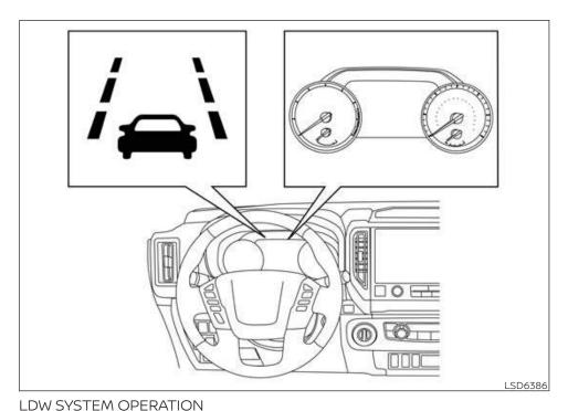
The LDW system provides a lane departure warning function when the vehicle is driven at speeds of approximately 37 mph (60 km/h) and above and the lane markings are clear. When the vehicle approaches either the left or the right side of the traveling lane, the steering wheel will vibrate and the LDW indicator on the instrument panel will blink to alert the driver.
