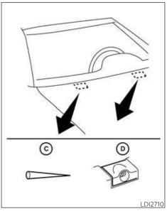
Be careful not to let anything get into the washer nozzle (1). This may cause clogging or improper windshield-washer operation. If something gets into the nozzle, remove it with a needle or small pin (3).
