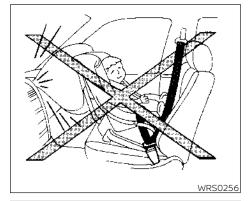
Even with the NISSAN Advanced Air Bag System, never install a rearfacing child restraint in the front seat. An inflating front air bag could seriously injure or kill your child. For additional information, see "Child restraints" (P. 35).
