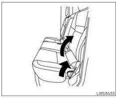
1. Lift up on the lever, located on the side of the seat, while lifting the front of the seat cushion up.
