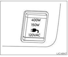
To use the outlets for devices that require up to 120v power, the vehicle must be running and the power inverter switch must be on.
