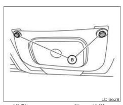
Oil filter access cover (Type A) (if so equipped)
