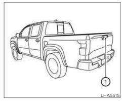
To display the rear view, the Rear View Monitor system uses a camera located just above the vehicle's license plate 1 on the tailgate.
