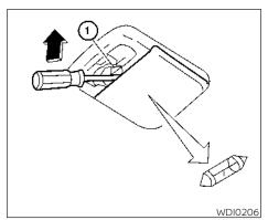
**Room light (Type A) (if so equipped)**Use a cloth (1) to protect the housing.
