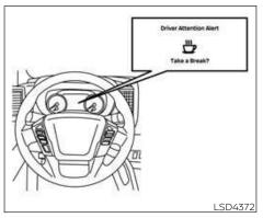
The system resets and starts reassessing driving style and steering behavior when the ignition switch is cycled from the ON to the OFF position and back to the ON position.
