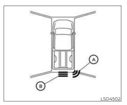
When the corner of the vehicle moves closer to an object, the corner sonar indicator  ${\Large \textcircled{\sc A}}$  appears. When the center of the vehicle moves close to an object, the center sonar indicator (B) appears.
