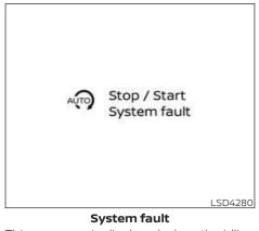
This message is displayed when the Idling Stop System is malfunctioning.
