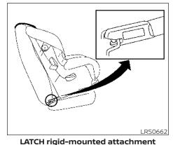
LATCH compatible child restraints include two rigid or webbing-mounted attachments that can be connected to two anchors located at certain seating positions in your vehicle. With this system, you do not have to use a vehicle seat belt to secure the child restraint. Check your child restraint for a label stating that it is compatible with LATCH. This information may also be in the instructions provided by the child restraint manufacturer.
