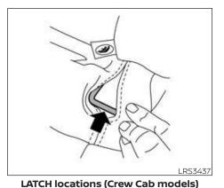
The LATCH lower anchors are located as shown. A label is attached to the seatback to help you locate the LATCH lower
