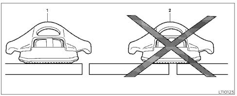
1 correct installation, 2 incorrect installation
