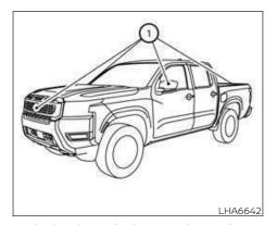
To display the multiple views, the Intelligent Around View® Monitor system uses cameras located in the front grille, on the vehicle's outside mirrors and one on the tailgate ①.
