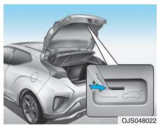
Your vehicle is equipped with an emergency tailgate safety release lever located on the bottom of the tailgate inside the vehicle.
