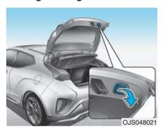
Lower the tailgate lid and press down until it locks. To be sure the tailgate lid is securely fastened, always check by trying to pull it up again without pressing the tailgate handle button.
