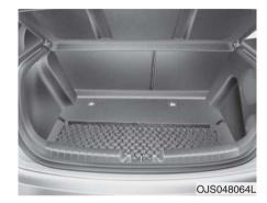
To keep items from shifting in the cargo area, you can use the four hooks located in the cargo area to attach the luggage net.
