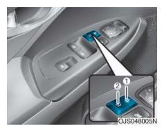
The driver side door armrest is equipped with a central door lock switch. The lock button is indicated by a (1) symbol. The unlock button is indicated by a (1) symbol.
