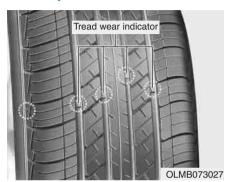
If the tire is worn evenly, a tread wear indicator will appear as a solid band across the tread. This shows there is less than 1.6 mm (2/32 inch) of tread left on the tire. Replace the tire when this happens.
