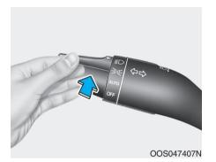
To turn on the high beam headlamp, push the lever away from you. The lever will return to its original position. The high beam indicator will light when the headlamp high beams are switched on.
