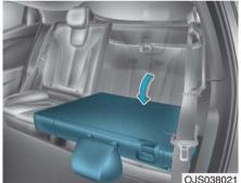
4. Remove the belt from the clip (1) and pull up the seatback folding lever (2), then fold the seat toward the front of the vehicle.
