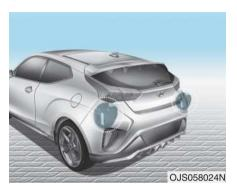
The sensors are located inside the rear bumper.
