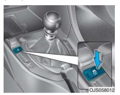
The Electronic Stability Control (ESC) system helps to stabilize the vehicle during cornering maneuvers. ESC checks where you are steering and where the vehicle is actually going. ESC applies braking pressure to any one of the vehicle's brakes and intervenes in the engine management system to assist the driver with keeping the vehicle on the intended path. It is not a substitute for safe driving practices. Always adjust your speed and driving to the road conditions.
