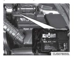
Inside the fuse/relay box cover, you can find the fuse/relay label describing fuse/relay names and ratings.
