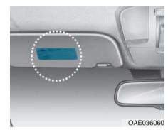
Air bag warning labels, required by the Canadian Motor Vehicle Safety Standards (CMVSS), are attached to alert the driver and passengers of potential risks of the air bag system. Be sure to read all of the information about the air bags that are installed on your vehicle in this Owners Manual.
