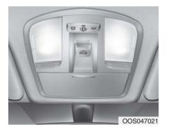
The sunroof can only be opened, closed, or tilted when the ignition switch is in the ON position.
