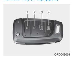
Your HYUNDAI uses a remote key, which you can use to lock or unlock the driver and passenger doors or the rear tailgate.
