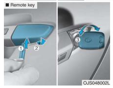
If you lock the driver's door with a mechanical key, all vehicle doors will lock.
