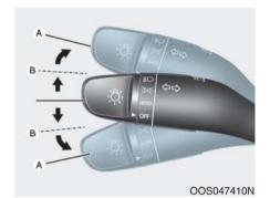
To signal a turn, push down on the lever for a left turn or up for a right turn in position (A).
