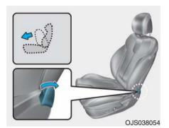
To get in or get out of the driver's door from the rear seat, the driver's seat should be folded by pulling the lever toward the rear of the vehicle.
