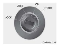
Whenever the front door is opened, the ignition switch will illuminate, provided the ignition switch is not in the ON position. The light will go off immediately when the ignition switch is turned on or go off after about 30 seconds when the door is closed. (if equipped)
