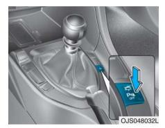
Push the button to turn OFF the Parking Distance Warning (Reverse) system. The indicator light on the button will turn on.
