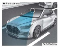
In order for the FCA system to operate properly, always make sure the camera is clean and free of dirt, snow, and debris.
