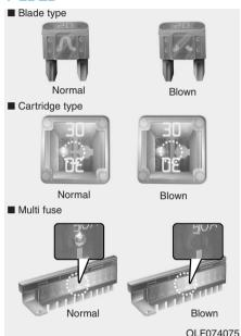
A vehicle's electrical system is protected from electrical overload damage by fuses.
