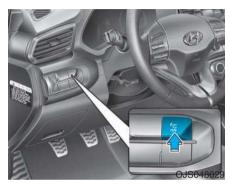
Use the button on the left hand side of the dash panel to activate/deactivate the Head-up display when the ignition is in the ON position or when the engine is running.
