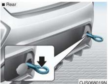
If towing is necessary, we recommend you have it done by an authorized HYUNDAI dealer or a commercial tow truck service. If a towing service is not available in an emergency, your vehicle may be temporarily towed using a cable or chain secured to the emergency towing hook at the front (or rear) of the vehicle.
