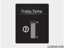
The transmission temperature gauge display shows the current temperature of the dual clutch transmission.
