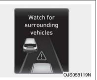
If the vehicle ahead (vehicle speed: less than 30 km/h (20 mph)) disappears to the next lane, the warning chime will sound and a message "Watch for surrounding vehicles" will appear. Adjust your vehicle speed for vehicles or objects that can suddenly appear in front of you by depressing the brake pedal.
