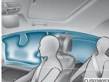
Curtain air bags are located along both sides of the roof rails above the front and rear doors. They are designed to help protect the heads of the front seat occupants and the rear outboard seat occupants in certain side impact collisions.
