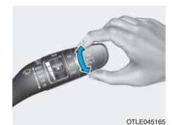
The rear window wiper and washer switch is located at the end of the wiper and washer switch lever. Turn the switch to the desired position to operate the rear wiper and washer.
