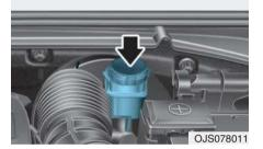
Check the fluid level in the reservoir periodically. The fluid level should be between MAX and MIN marks on the side of the reservoir.
