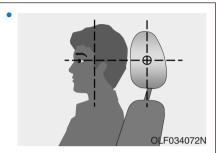
Adjust the head restraints so the middle of the head restraint is at the same height as the height of the top of the eyes.
