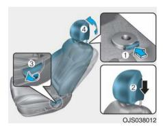
To reinstall the head restraint:
