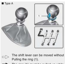
The ring (1) must be pulled up while moving the shift lever.
