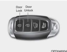
Press the button on the driver's outside door handle while carrying the Smart Key with you or press the Door Unlock button on the Smart Key, the driver's door will unlock.
