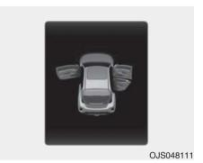
This warning is displayed if any door or the hood or the tailgate is left open. The warning will indicate which door is open in the display.
