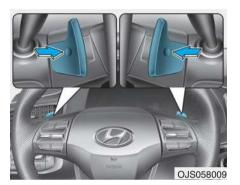
The paddle shifter is functional when the shift lever is in the D (Drive) position or the manual shift mode.
