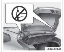
Do not hold on to or try to pull on the tailgate strut. Be aware that the deformation of the tailgate strut may cause vehicle damage and risk of injury.
