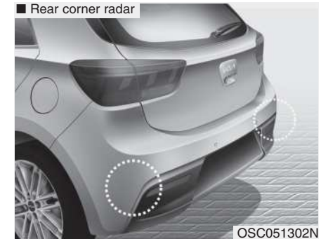
[A]: Rear Cross-Traffic Collision Warning operating range
